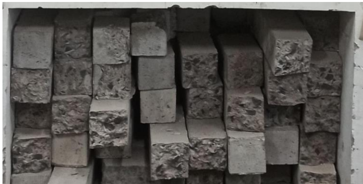
Fig. 5. SCC specimens after Flexural strength testing
