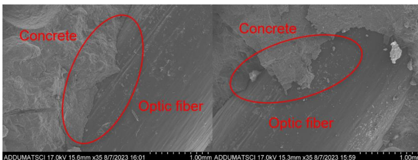
Fig. 13. Micro image of bond between concrete and fiber optic
