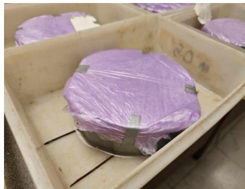
Fig. 7. Samples underwent in capillary absorption test
