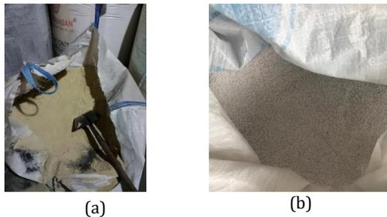
Fig. 2 Used binders (a) bentonite and (b) perlite
