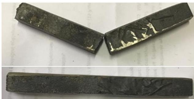
Fig. 6 Three-point bending test samples
