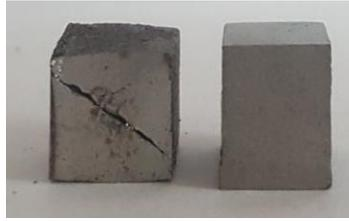
Fig. 9 Fractured samples after tensile- compression test
