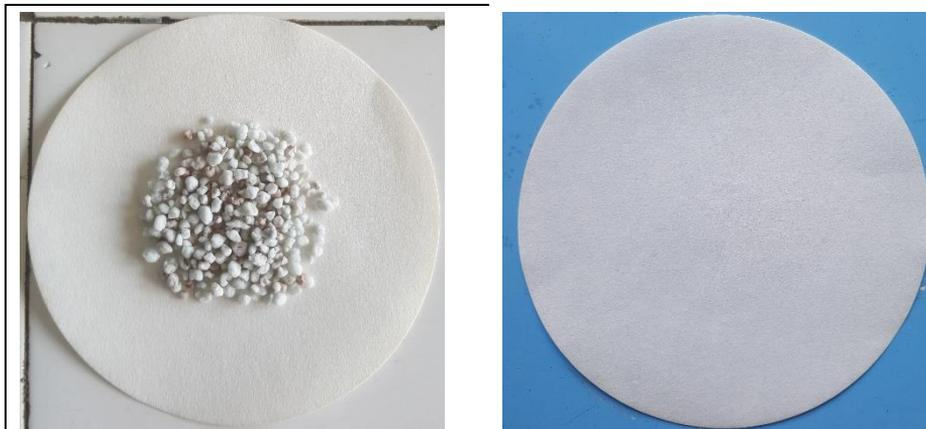
Figure 2. Images of the leakage test of the composite PCM
