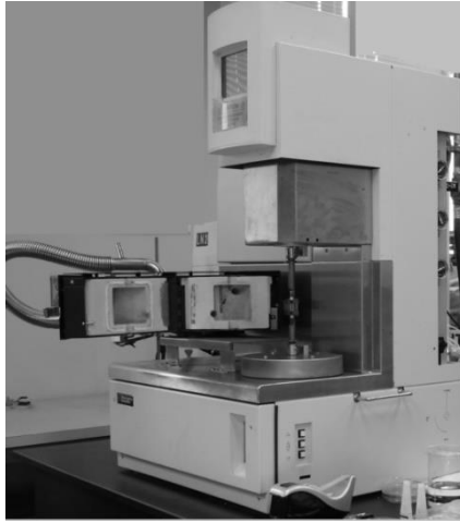
Fig. 1 Computer Automated Dynamic Thermo-Mechanical Analyzer (Entire System)
