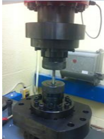
Fig. 1 Zwick HA 250kN hydraulic fatigue testing machine
