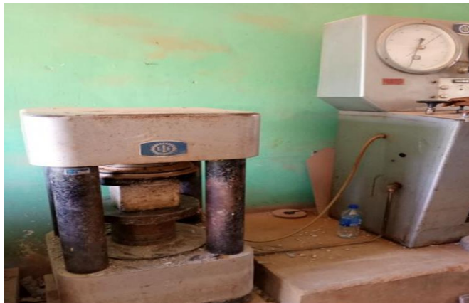
Fig. 3 Destructive Compression Test on Concrete Samples
