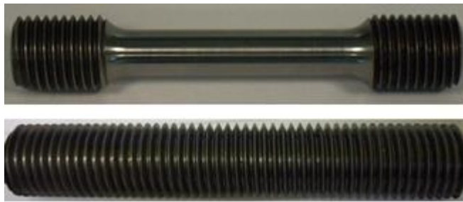
Fig. 2 Fatigue specimens and original screwed bar
