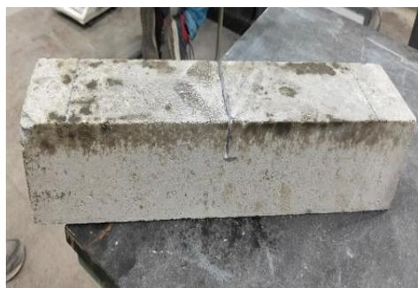
Fig. 4 Notched beam sample
