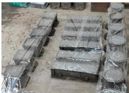
Fig. 3 Concrete cubes, cylinders, and beams in molds
