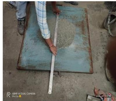
Fig. 8 Slump flow test
