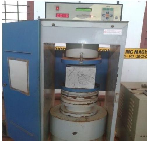
Fig. 1 Test setup for compressive strength
