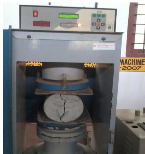
Fig. 2 Test setup for split tensile strength
