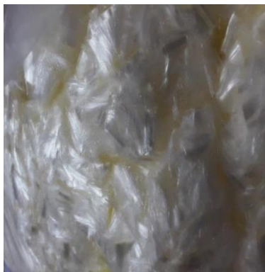
Fig. 4 Treated (or) Oiled PVA fibres
