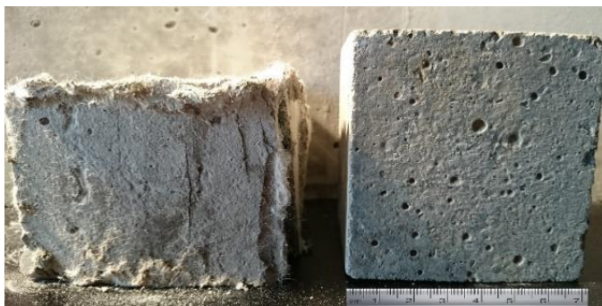
Fig. 1 ECC high ability to withstand compression
