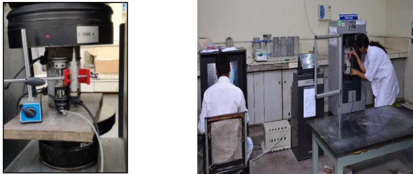
Fig. 3 Testing setup for Stress Strain Curve determination
