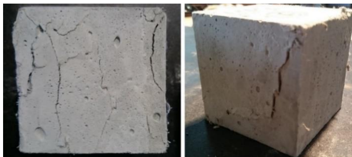
Fig. 2 Cracking pattern in ECC specimens due to compressive test
