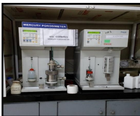
Fig. 1 Test setup for evaluation of pore structure
