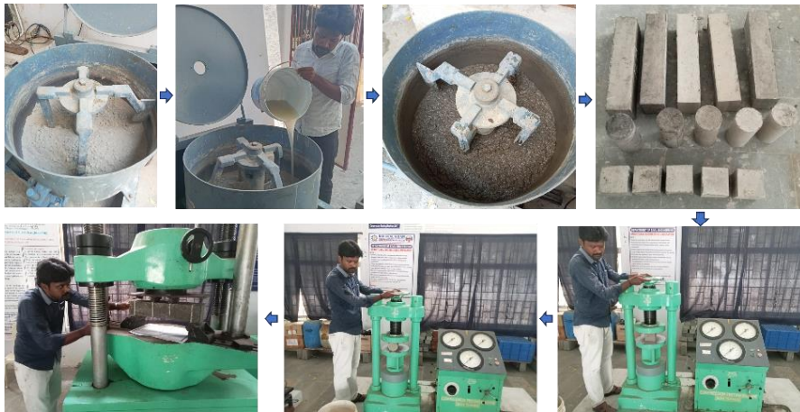
Fig. 5 Specimens preparation and test setup of compression (cube), split tensile (cylinder) and flexural (prism)
