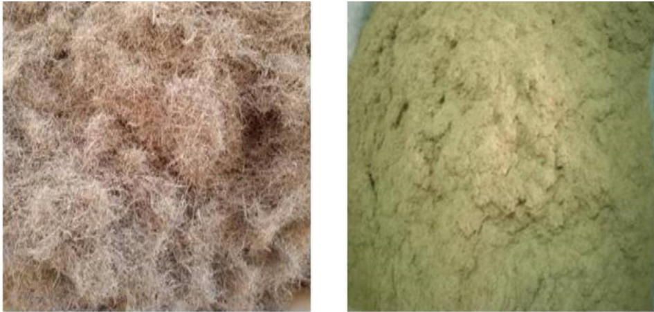
Fig. 2 Fibers from Posidonia Oceanica after crushing and sieving
