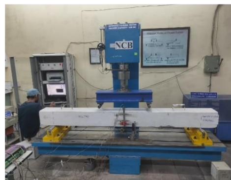
Fig. 8 Test Configuration for Beams [55]
