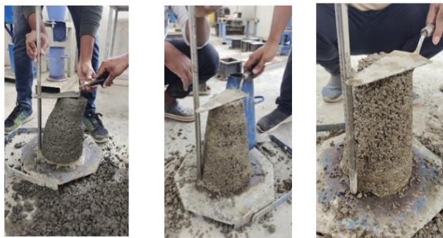
Fig. 7 Slump pattern of different concrete mix
