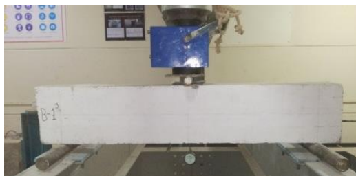
Fig. 6 Test setup and testing of beam
