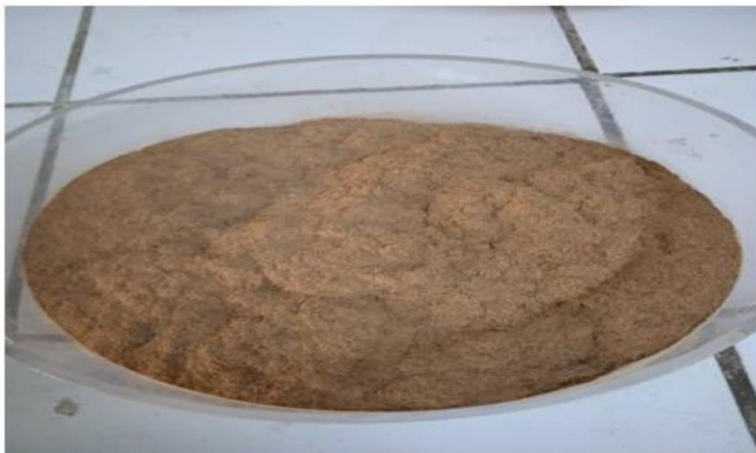
Fig. 3 Fibers treated and coated with calcined clay
