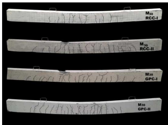
Fig. 10 RCC and GPC Beam Crack Pattern [52]
