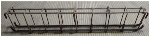
Fig. 2 Details of reinforcements of beam
