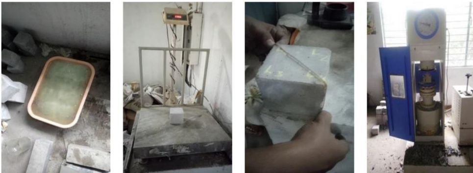
Fig. 3 Experimental setup for acid attack test
