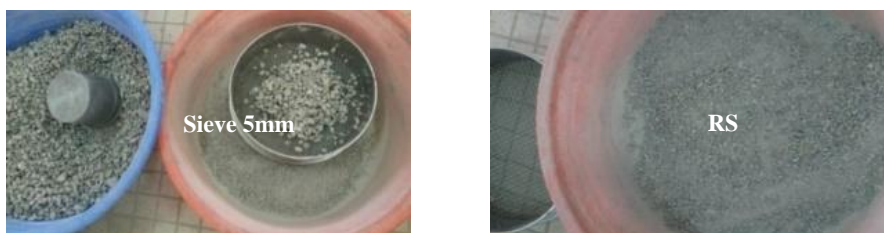
Fig. 1 Preparation of recycled sand by sieving
