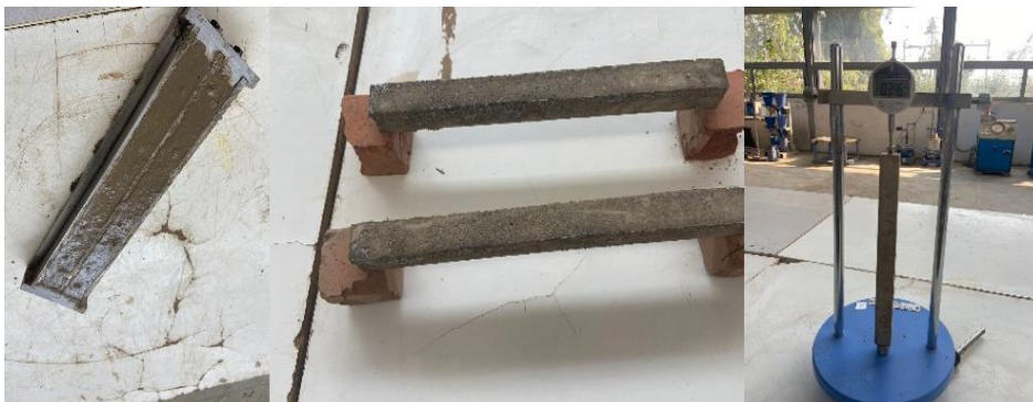
Fig. 5 Drying shrinkage test using length comparator
