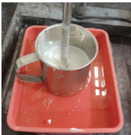
Fig. 4 Dispersion of Nano-clay in unsaturated polyester resin
