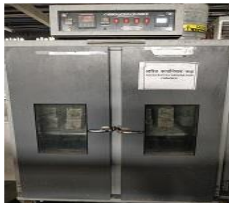
Fig. 2 Accelerated Carbonation Test
