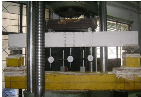
Fig. 6 Test Arrangement for Flexure [54]
