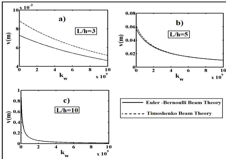
Fig. 3. The effect of Winkler spring constant ( $k_w$ ) on the maximum vertical displacements of the FG beam for different slenderness ratio ( $L/h$ ), a)  $L/h=3$ , a)  $L/h=5$  and a)  $L/h=10$ .
