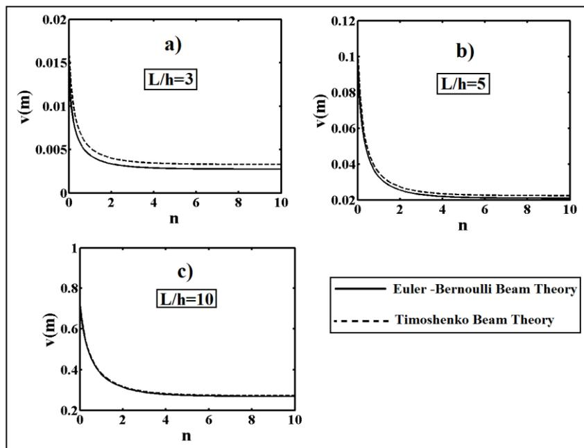
Fig. 2. The effect of material distribution ( $n$ ) on the maximum the vertical displacements of the FG beam for different slenderness ratio ( $L/h$ ), a)  $L/h=3$ , a)  $L/h=5$  and a)  $L/h=10$ .
