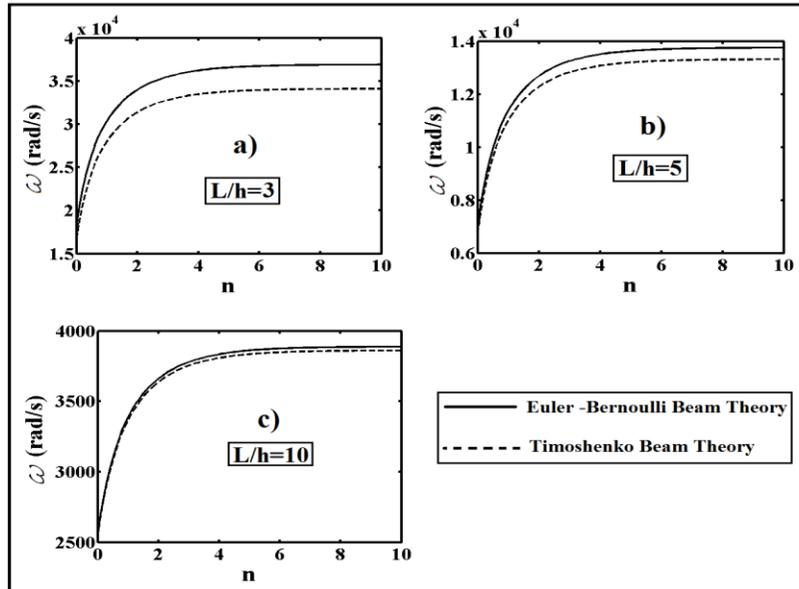
Fig. 4. The effect of material distribution ( $n$ ) on the maximum the fundamental frequency ( $\omega$ ) of the FG beam for different slenderness ratio ( $L/h$ ), a)  $L/h=3$ , a)  $L/h=5$  and a)  $L/h=10$ .
