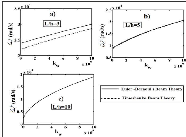
Fig. 5. The effect of Winkler spring constant ( $k_w$ ) on the fundamental frequency ( $\omega$ ) of the FG beam for different slenderness ratio ( $L/h$ ), a)  $L/h=3$ , a)  $L/h=5$  and a)  $L/h=10$ .
