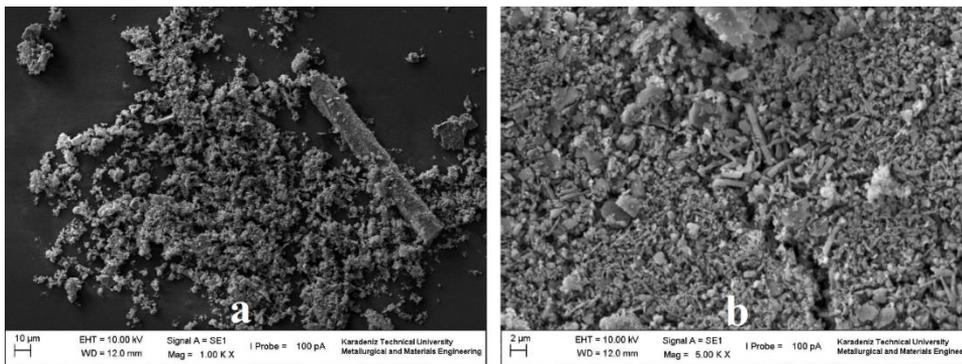
Fig. 11 SEM images of the debris of the sample seven (a-1000x, b-5000)
