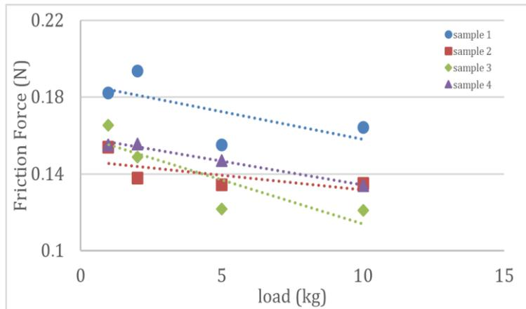
Fig. 12 Friction force versus load diagram of the constant pressure samples
