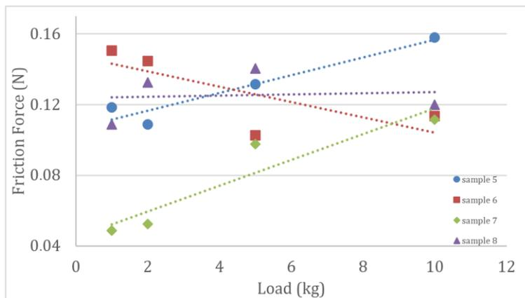
Fig. 13 Friction force versus load diagram of the constant temperature samples
