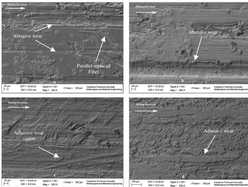
Fig. 9 SEM images of wear surface at constant pressure samples (500x) (a-1, b-2, c-3, d-4)
