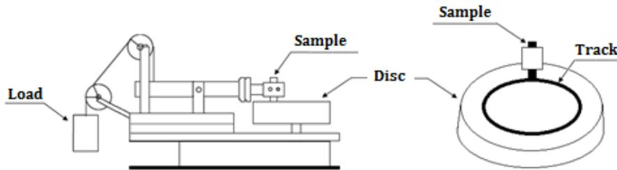
**Fig. 2 Schematic drawing of the pin-on-disc test machine**
