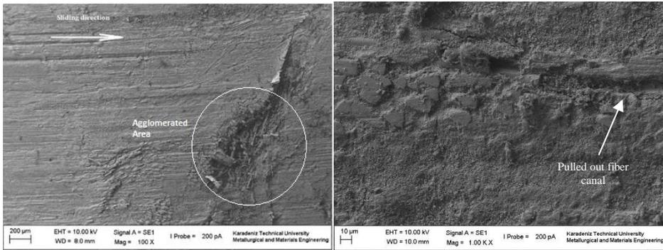
Fig. 8 a) Agglomerated fiber SEM image of the sample six (100x) b) Pulled out fiber canal of the sample four (1000x)
