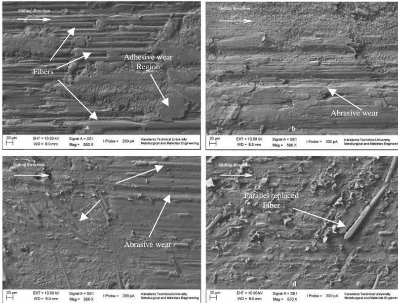
Fig. 10 SEM images of wear surface at the constant temperature samples (500x) (a-5, b-6, c-7, d-8)
