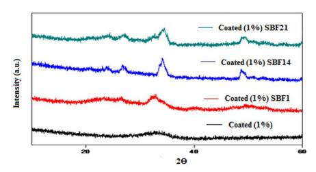
Fig. 10 XRD patterns of 1% gelatine coated scaffolds before (a) and after (b) 1, (c) 14 and (d) 21 days immersion in SBF
