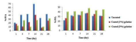
Fig. 13 (a) water absorption and (b) weight loss values for uncoated and coated scaffolds after immersion in SBF for 1, 4, 7, 14, 21 and 28 days
