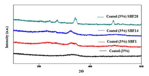
Fig. 11 XRD patterns of 3% gelatine coated scaffolds before (a) and after (b) 1, (c) 14 and (d) 28 days immersion in SBF
