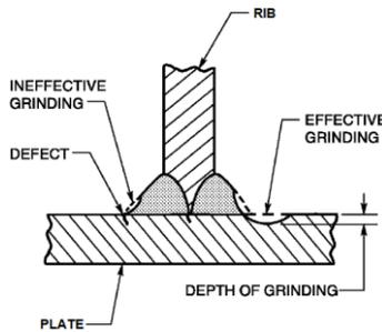
Fig. 3 Geometrical aspects related to toe grinding process [15]
