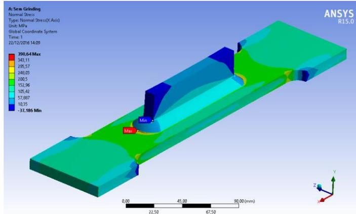
Fig. 11 Post-processing image obtained for the no-grinding case.
