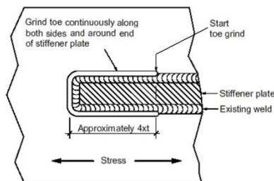
Fig. 5 Recommended contouring toe-grinding [11]
