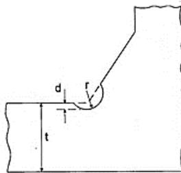
Fig. 4 Geometrical parameters related to toe grinding process [11]
