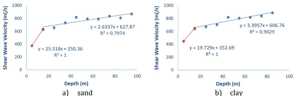
Fig. 1 Average shear wave depth velocity relation for sand and clay
