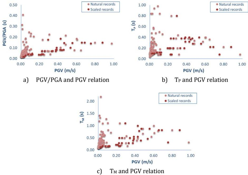
Fig. 2 The relationships between intensity and frequency content parameters for the scaled and natural earthquakes
