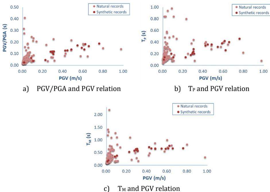
Fig. 3 The relationships between intensity and frequency content parameters for the synthetic and natural earthquakes
