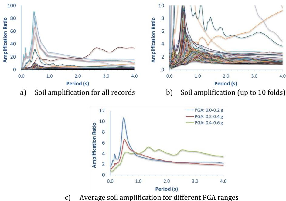
Fig. 4 Soil amplification values for all 84 records and averages for different PGA ranges
