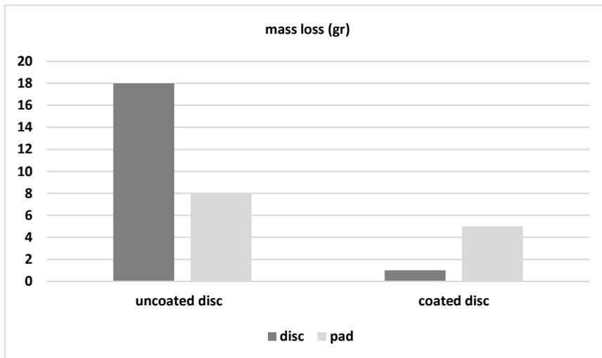
Fig. 6 Comparative mass loss of APS Al<sub>2</sub>O<sub>3</sub>-TiO<sub>2</sub> coated and uncoated brake discs and corresponding pad mass loss
