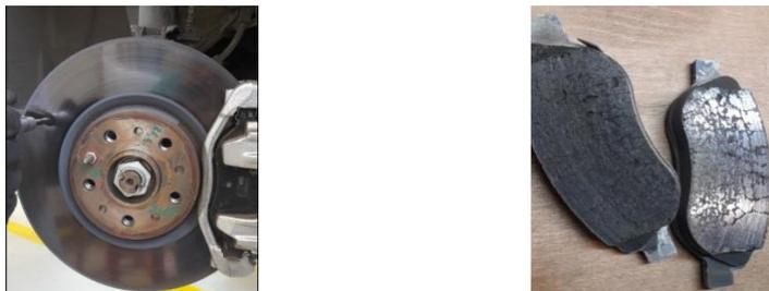
Fig. 4 Disc and pad surface photographs after vehicle road test
