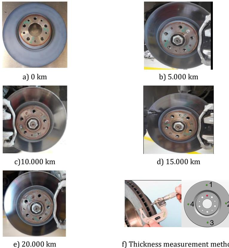
Fig. 3. On vehicle test: plasma spray coated disc images and measurement method
