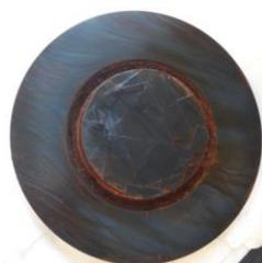
Fig. 5 Coated disc brake surface after salt spray corrosion test
