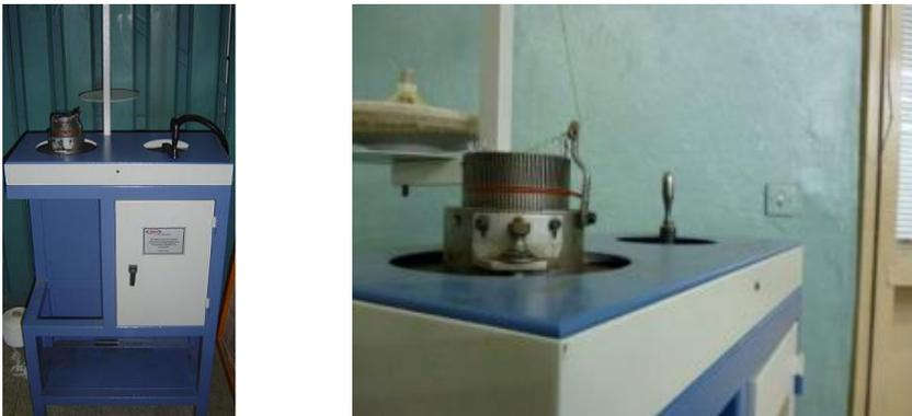
Fig. 3. Mechanical single jersey circular knitting machine.
