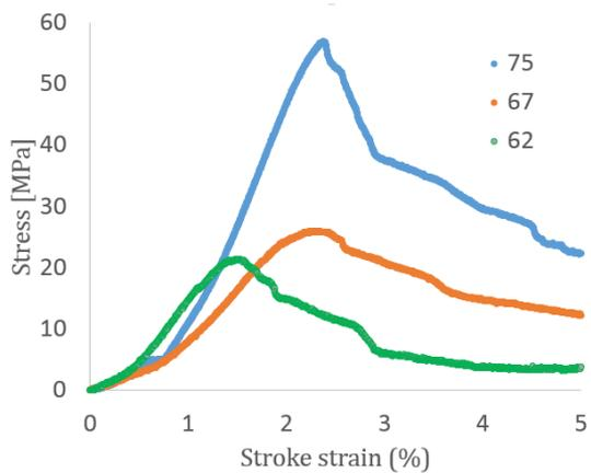
Fig. 8. Typical stress-strain graphs for the compression tests of braided tubes.
