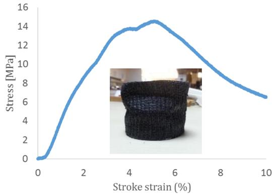
Fig. 7. Typical stress-strain graph for the compression test of knitted tubes.
