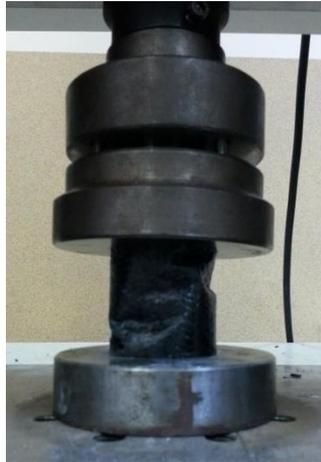
Fig. 9. Diamond shaped buckling of braided tubes during compression testing.
