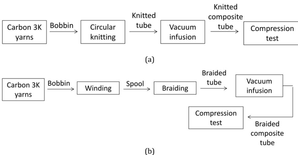
Fig. 6. Methodology of the experiments for the circular knitted composite tubes (a), and the braided composite tubes (b).
