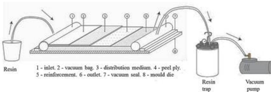
Fig. 4. Typical vacuum infusion lay-up components [23]
