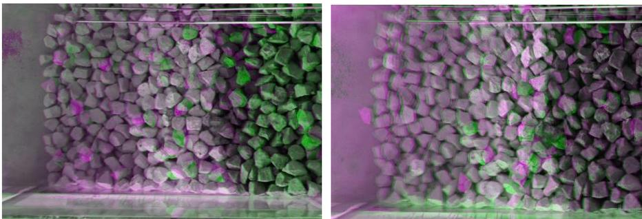
Fig. 8 Left: Differences between photos taken before Test 10 and after Test 16.
