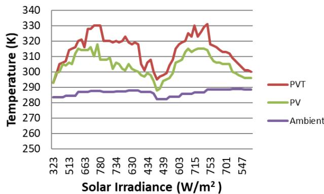
Fig 3. Variation of surface temperature (K) of PV and PVT systems and ambient temperature (K)
