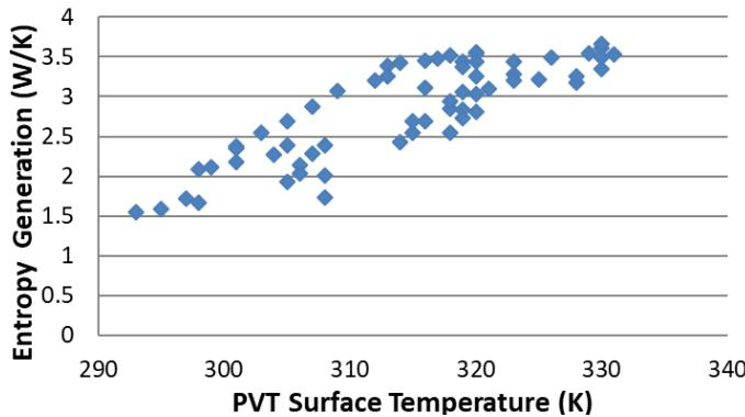
Fig 7. Variation of the entropy generation (W/K) of the PVT system due to surface temperature of PVT system
