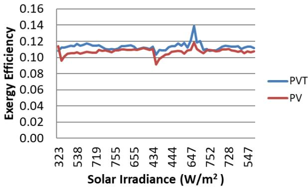
Fig 5. Variation of the exergy efficiency of PV and the PVT system due to solar irradiance ( $\text{W/m}^2$ )
