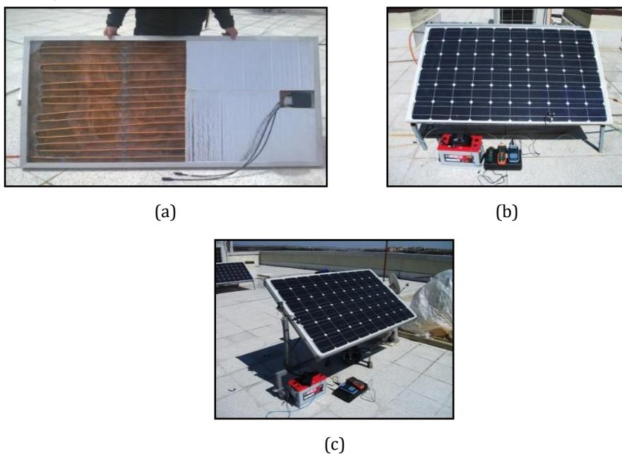
Fig 1. The photos of the experimental set up (a) Structure of PVT system, (b) Obtaining data for PVT system, (c) Obtaining data for PV system
