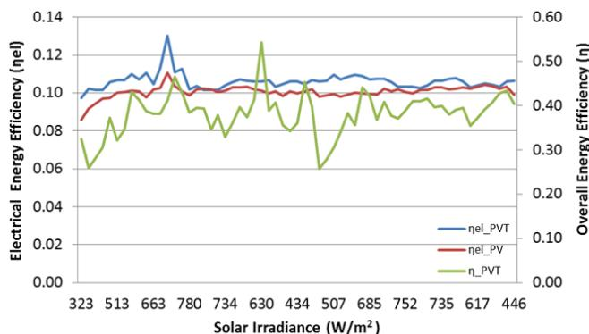
Fig 4. Variation of the electrical energy efficiency of PV and the PVT system and overall energy efficiency of the PVT system due to solar irradiance (W/m²)
