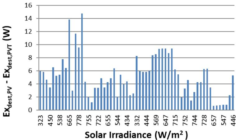
Fig 6. The difference of the exergy destruction (W) of the PV system and PVT system by solar irradiance ( $\text{W/m}^2$ )
