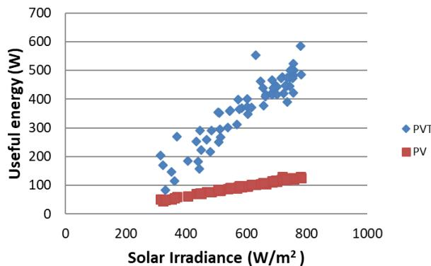
Fig 2. Variation of the useful energy rate (W) obtained from the PV and the PVT systems by solar irradiance ( $\text{W/m}^2$ )
