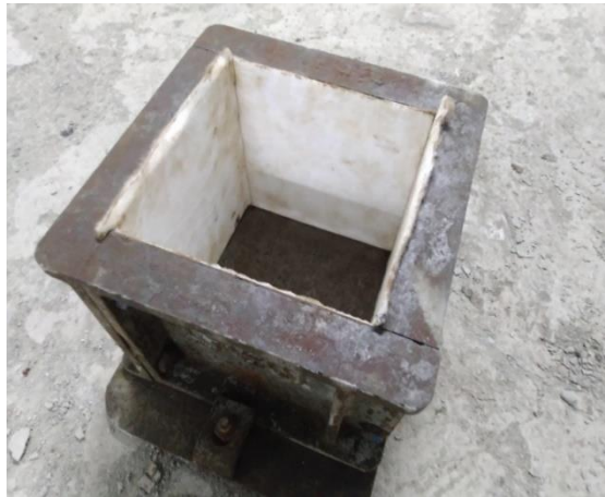
Fig. 2 Steel Mould with CPF Liner Pasted Inside
