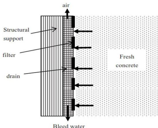
Fig. 1 Factors of a CPF System [8]
