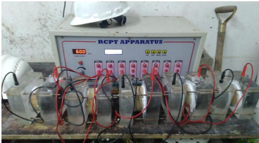
Fig. 4 RCPT Apparatus with Specimens
