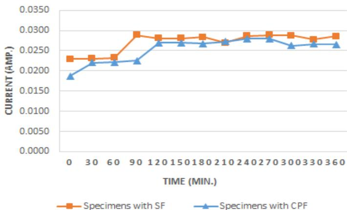
Fig. 8 Current Vs Time for RCPT Test
