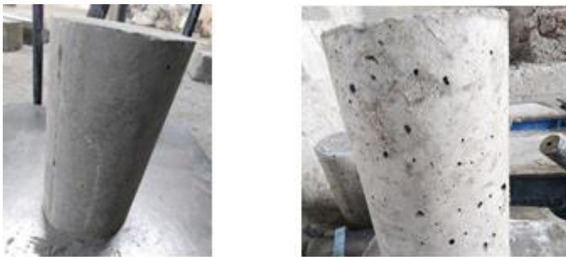
Fig. 6 Surface of Demoulded Cylindrical Specimens
