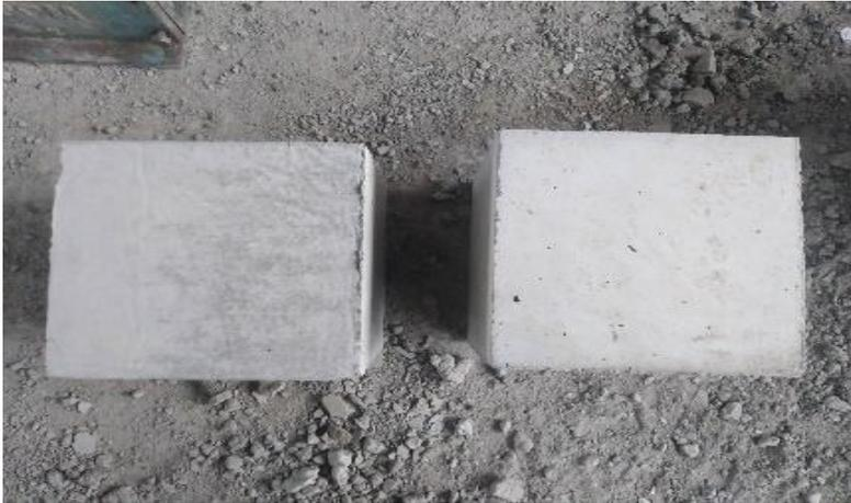
Fig. 5 Surface of Demoulded Cubic Specimens
