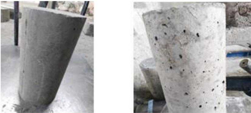
Fig. 6 Surface of Demoulded Cylindrical Specimens
