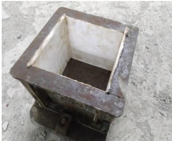
Fig. 2 Steel Mould with CPF Liner Pasted Inside
