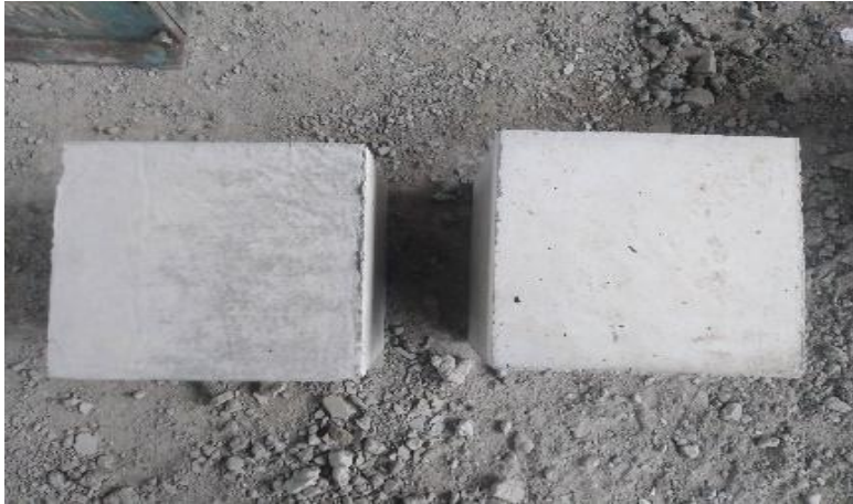
Fig. 5 Surface of Demoulded Cubic Specimens
