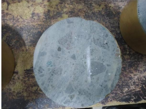
Fig. 3 Core Sample From Specimen for RCPT
