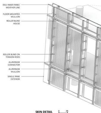
Fig 2 Triple Glazed Detail [7]
