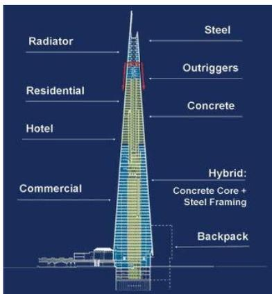
Fig. 4 Construction Technique and Usage Functions According to Shard Floors, Cambridge [9]
