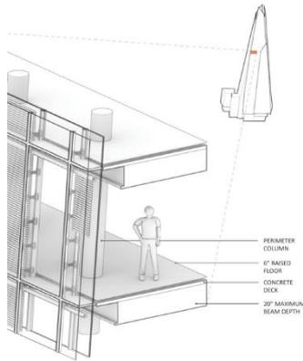
Fig. 3 The Shard Facade, Triple Glazed Detail [7]
