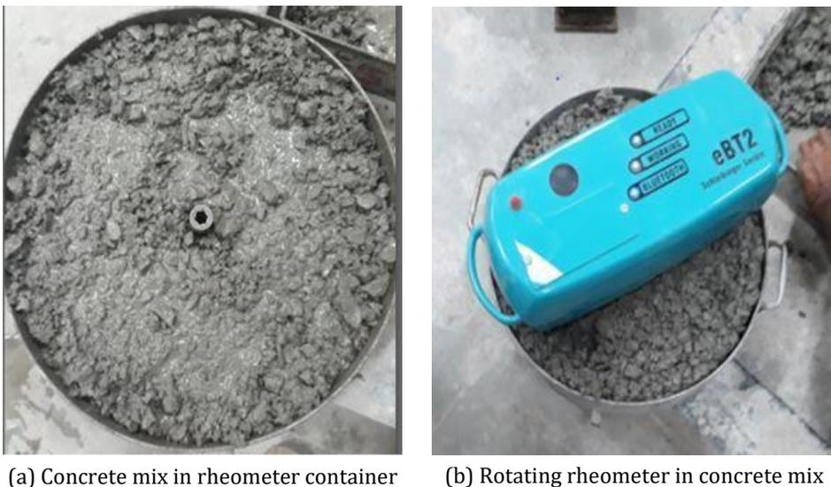
Fig. 3 Working of rheometer test apparatus
