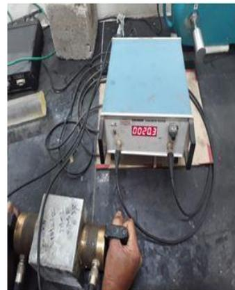
Fig. 5 Arrangement of Ultrasonic Pulse Velocity Test
