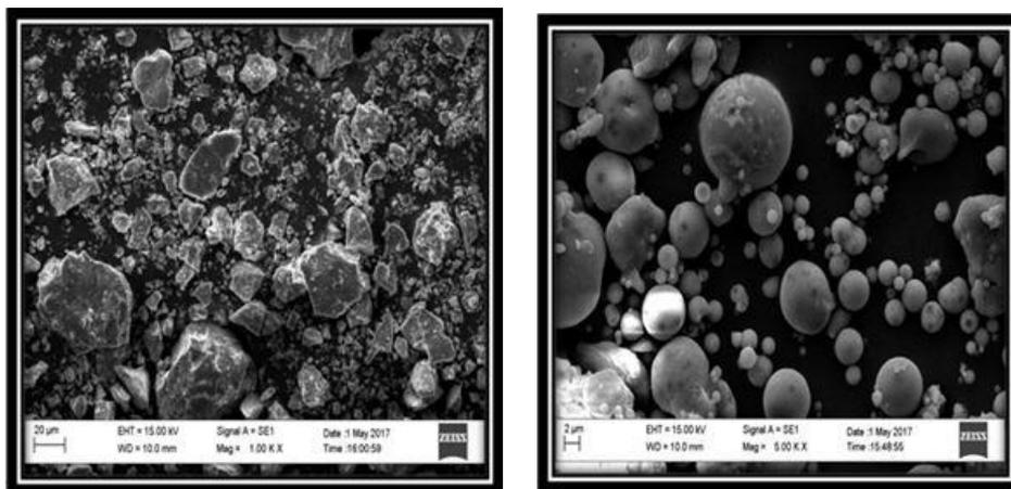
(a) SEM image of cement particles
