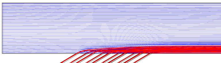
Fig.12 Velocity field streamlines along the solution domain for blowing ratio 1.5 at injection angle  $30^\circ$
