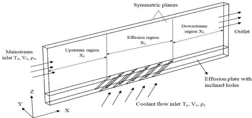
Fig. 1 Schematic of computational domain (XYZ)
