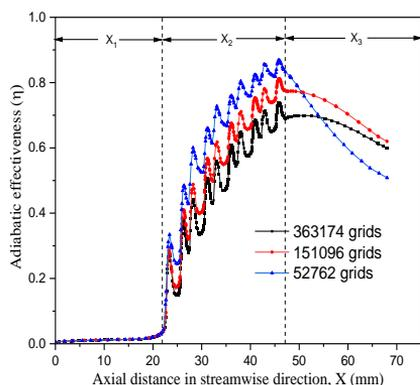
Fig. 4 Centerline adiabatic effectiveness on the effusion surface with different grid sizes for  $\alpha=30^\circ$  and  $BR=0.5$
