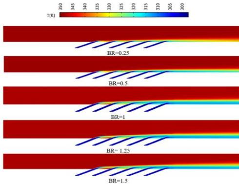
Fig. 7 Temperature slice counters on the center plane of effusion plate for different BR on XZ plane for  $\alpha=30^\circ$
