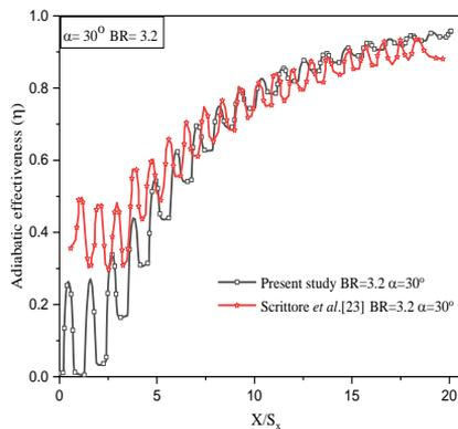
Fig. 5 Validation of experimental [23] and computational results. Note that the leading edge of first row  $X/S_x=0$  and adiabatic effectiveness is measured from rows 1 to 20
