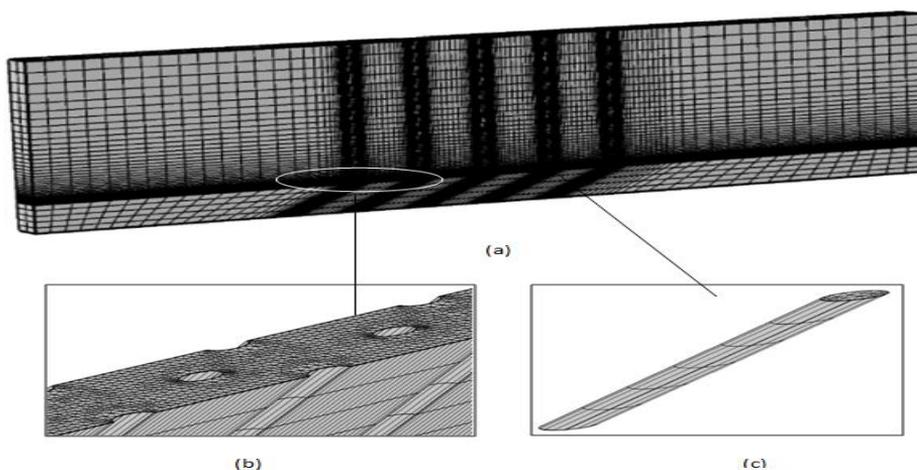
Fig. 3 Computational Mesh (a) Entire geometry (b) Effusion plate surface (c) Effusion hole
