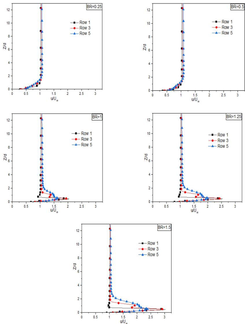
Fig.11 Velocity profiles downstream the effusion hole rows at different blowing ratios ( $\alpha=30^\circ$ )
