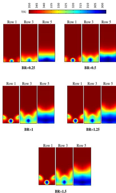
Fig. 13 Development of temperature fields on the YZ plane for different blowing ratios at  $\alpha=30^\circ$
