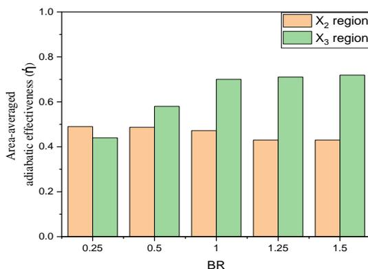
Fig. 16 Area-averaged adiabatic effectiveness ( $\bar{\eta}$ ) with blowing ratio (BR) in the effusion region ( $X_2$ ) and downstream region of effusion holes ( $X_3$ )
