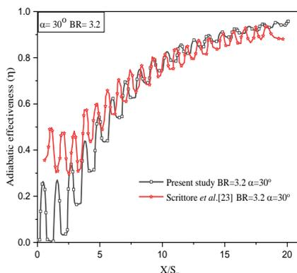
Fig. 5 Validation of experimental [23] and computational results. Note that the leading edge of first row  $X/S_x=0$  and adiabatic effectiveness is measured from rows 1 to 20
