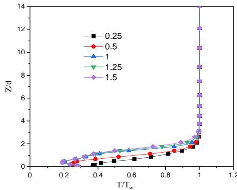
Fig. 14 Normalized Temperature boundary profiles at row 5 for  $\alpha=30^\circ$
