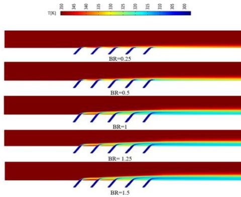
Fig.9 Temperature slice counters on the center plane of effusion plate for different BR on XZ plane for  $\alpha=60^\circ$
