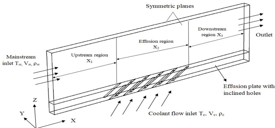
Fig. 1 Schematic of computational domain (XYZ)
