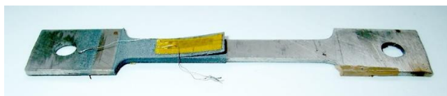
Fig. 12 Plasma-coated (Co-Cr alloy, thickness 160 \mu\text{m} ) Sample after tensile load test
