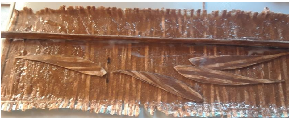
Figure 10 Placement of the Spar on the wing skin and image of the ribs
