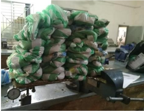
Figure 8 UAV wing subjected to loading using sandbags to determine its structural strength at the mechanical workshop, Bayero University Kano.
