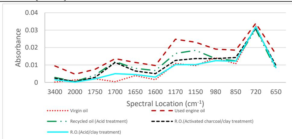
Fig. 7 FTIR Spectroscopic comparison of recycled oils
