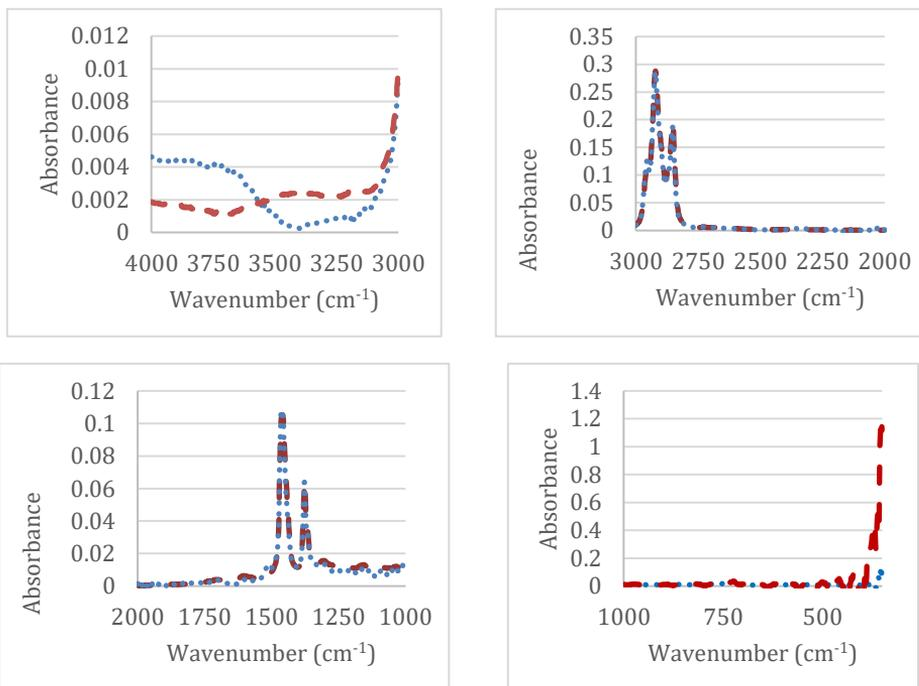
Fig. 4 FTIR of oil sample 4 from spectral location 4000 to 300  $\text{cm}^{-1}$  (red-used engine oil, blue- virgin oil)
