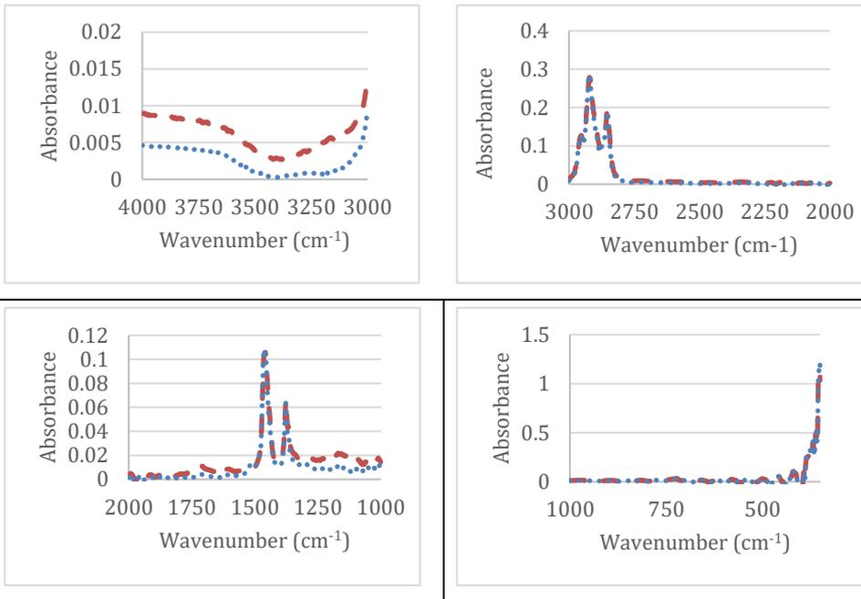
Fig. 2 FTIR of oil sample 2 from spectral location 4000 to 300 cm<sup>-1</sup> (red-used engine oil, blue- virgin oil)
