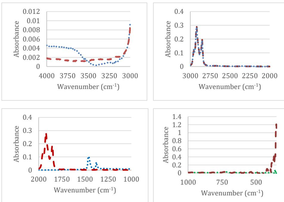
Fig. 5 FTIR of oil sample 5 from spectral location 4000 to 300  $\text{cm}^{-1}$  (red-used engine oil, blue- virgin oil)
