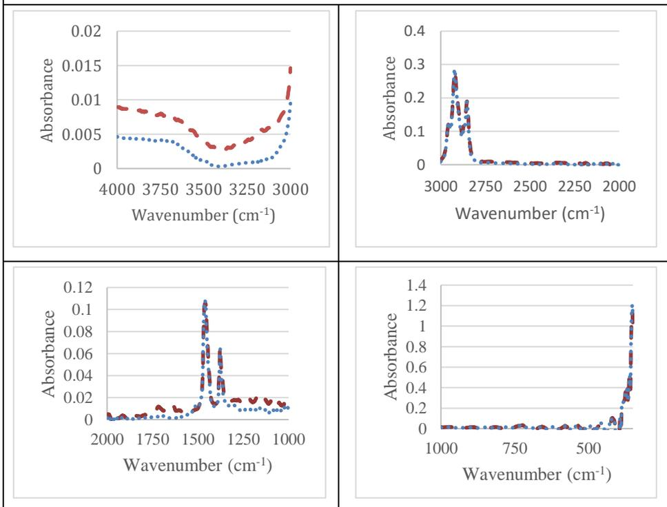
Fig. 3 FTIR of oil sample 3 from spectral location 4000 to 300 cm<sup>-1</sup> (red-used engine oil, blue- virgin oil)
