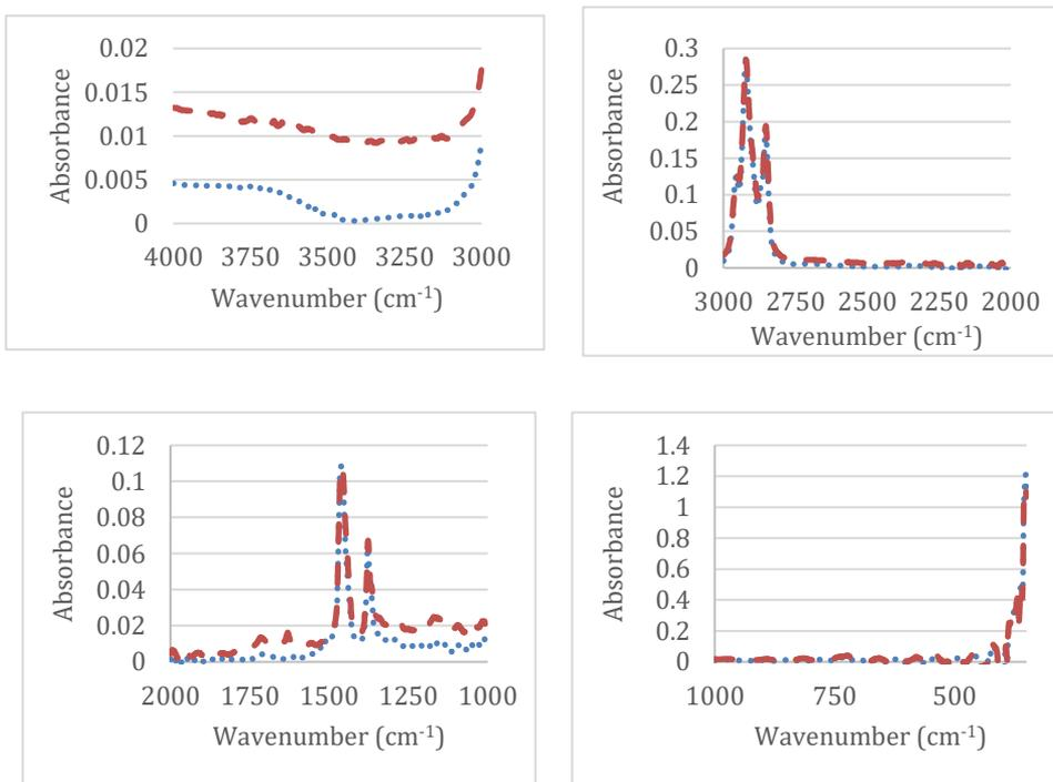
Fig. 1 FTIR of oil sample 1 from spectral locations 4000 to 300 cm<sup>-1</sup> (red-used engine oil, blue- virgin oil)
