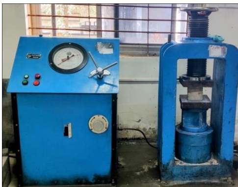
Fig.1 Testing arrangement for compressive strength test for concrete
