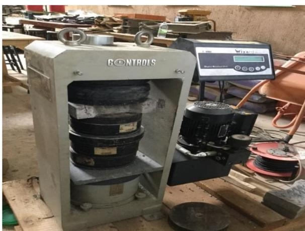
Fig. 2 Compressive strength setup
