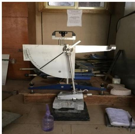
Fig. 3 Skid resistance test setup
