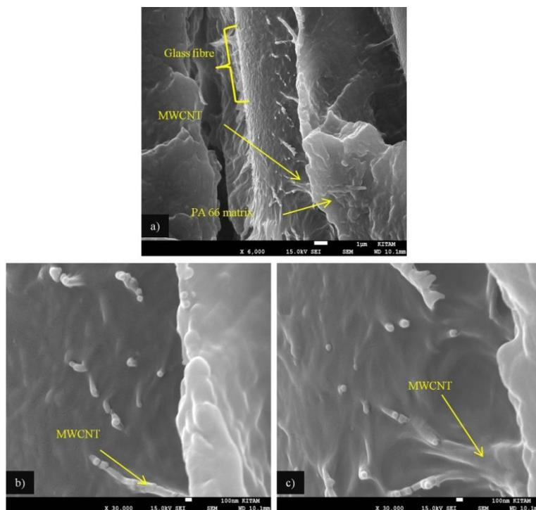
Fig. 7 SEM images of fractured MWCNTs-integrated PA 66/30SGF specimen
