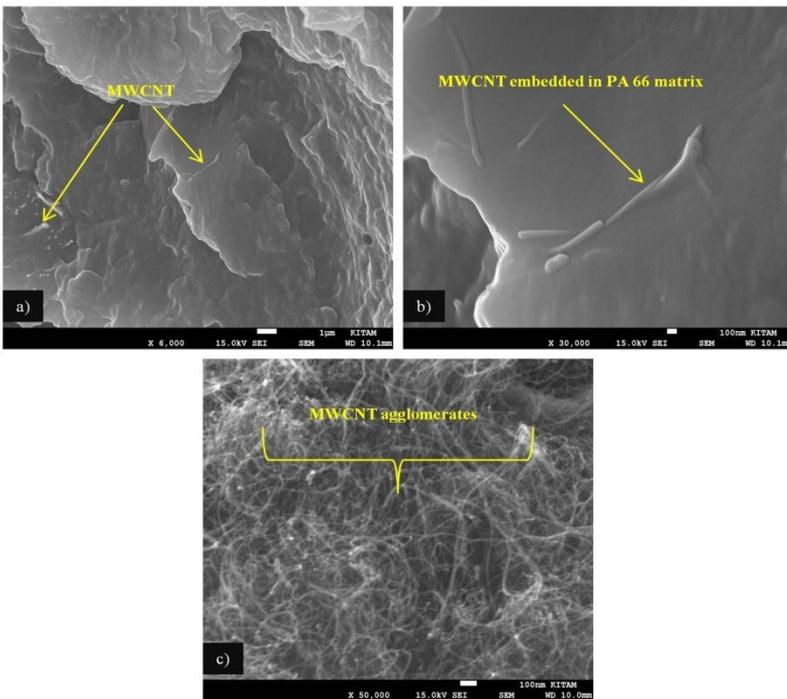
Fig. 9 SEM images of (a) MWCNTs embedded in PA 66/30SGF; (b) (higher-magnification) MWCNT embedded in PA 66/30SGF; (c) agglomerated MWCNTs
