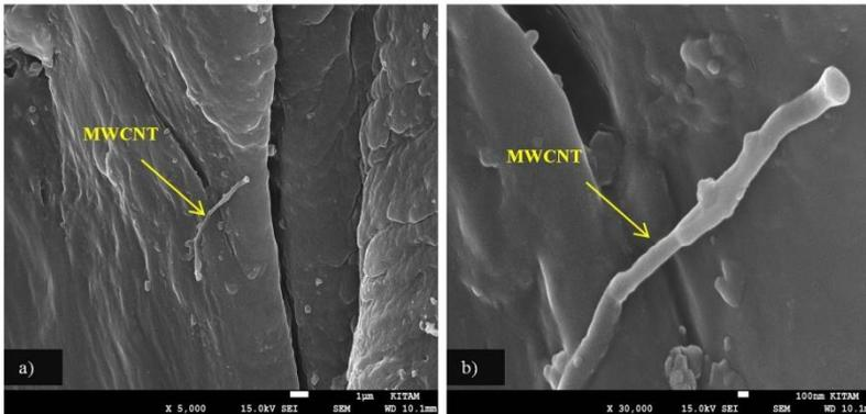
Fig. 8 SEM images of an individual MWCNT pull-out in a fractured PA 66/30SGF matrix
