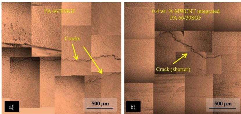
Fig. 6 Optical micrographs of fractured (a) PA 66/30SGF and (b) 0.4 wt.% MWCNT integrated PA 66/30SGF specimens monitored after 3-point flexural tests
