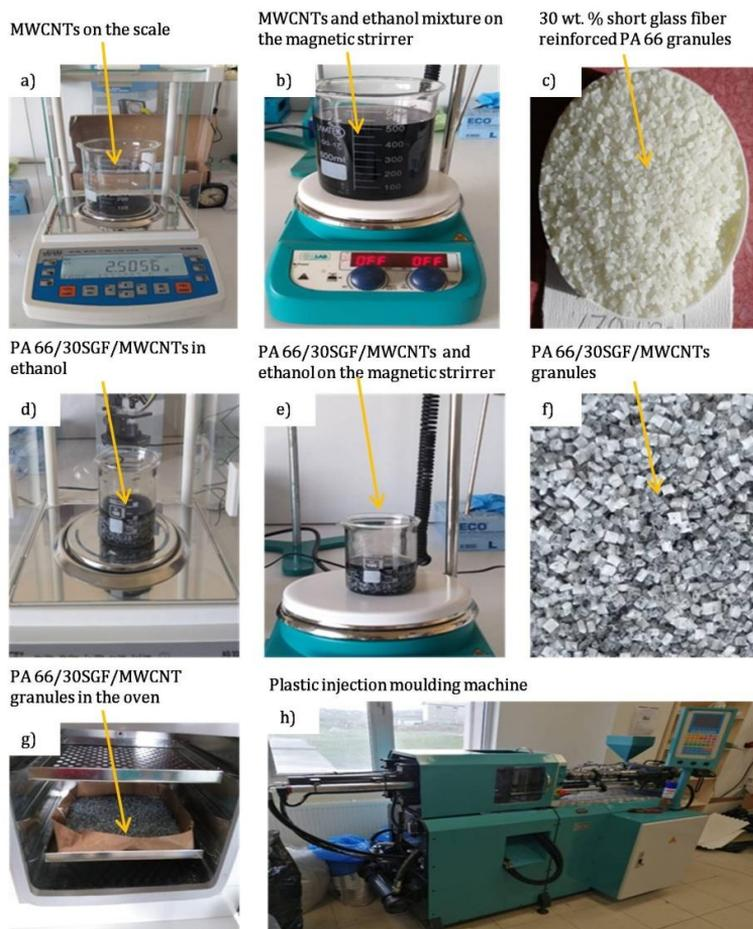
Fig. 1 Preparation process of PA 66/30SGF/MWCNT composite specimens
