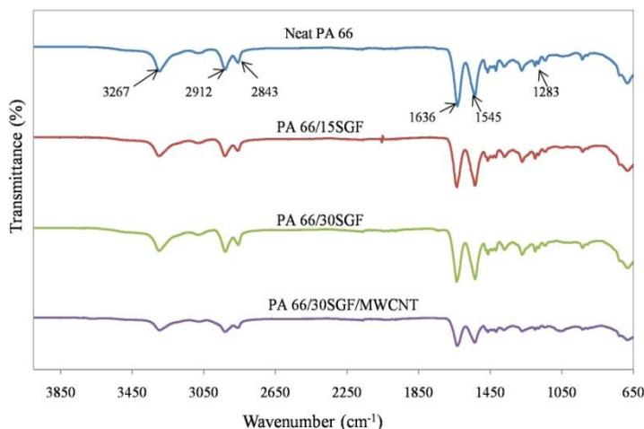
Fig. 3 FTIR spectra of the composite specimens
