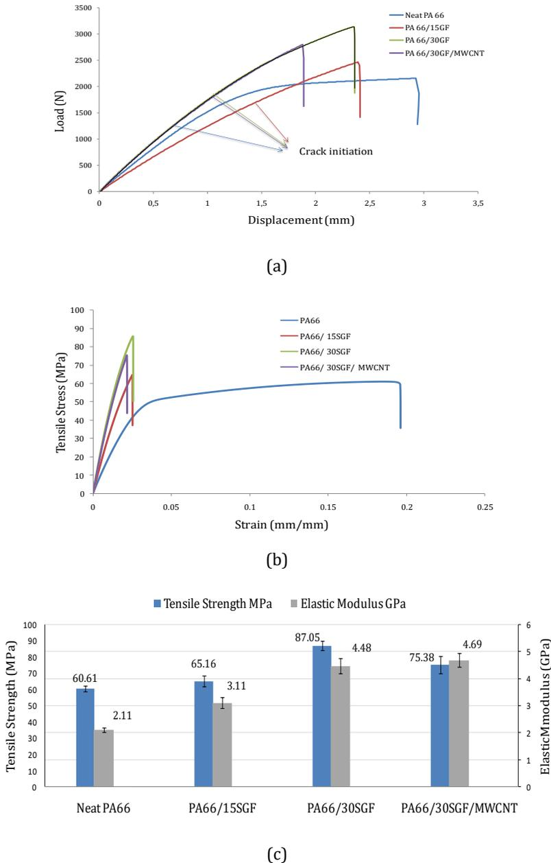
Fig.4 (a) Load-displacement curves of the specimens after the tensile tests; (b) Stress-strain curves of the specimens; (c) Tensile properties of the specimens
