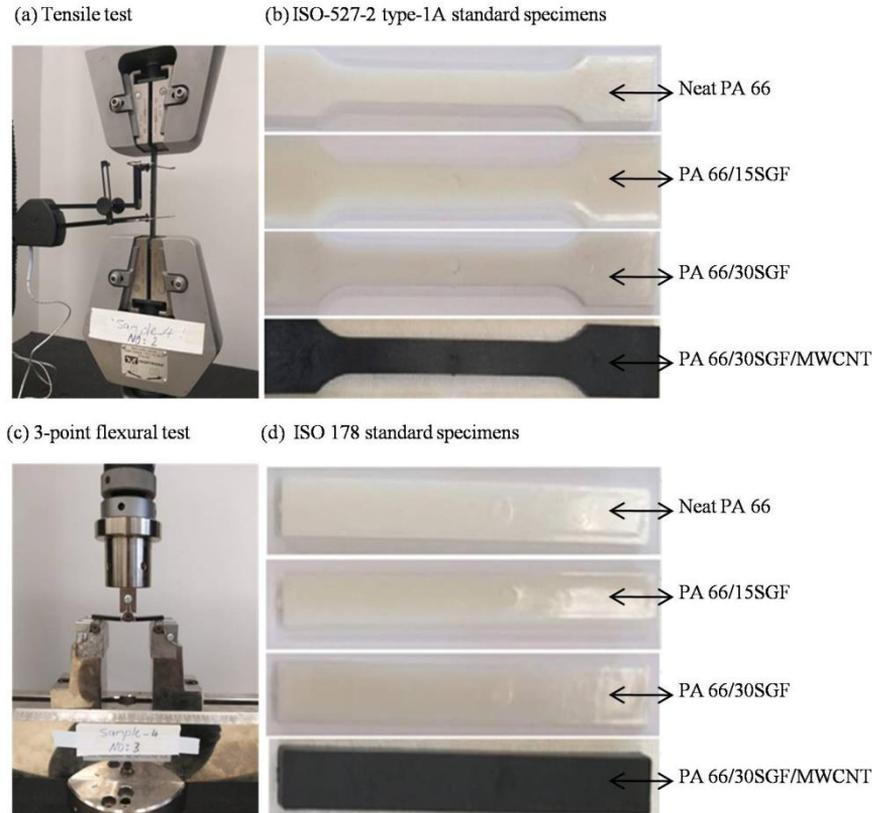
Fig. 2 Mechanical tests and specimens: (a) tensile test; (b) tensile test specimens in accordance with ISO 527-2 type-1A standard; (c) 3-point flexural test; (d) flexural test specimens in accordance with ISO 178 standard
