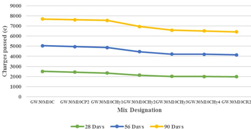
Fig. 8 Electrical resistivity value of various HFRGPC specimens
