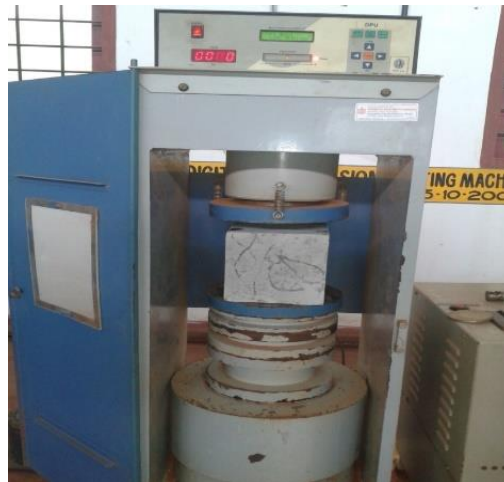
Fig. 1 Test setup for compressive strength
