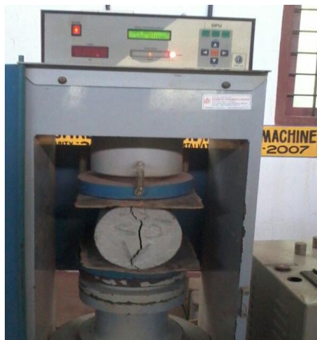
Fig. 2 Test setup for split tensile strength
