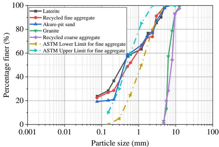
Fig. 2. The grain size distribution of aggregates
