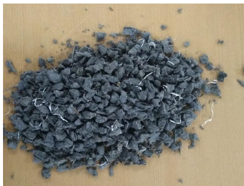
Fig. 1. Plastic wastes aggregate
