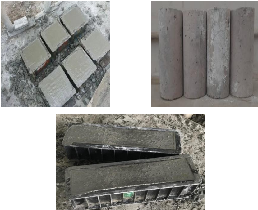
Fig. 2. Fabricated specimens (a) cube (b) cylindrical specimen and (c) rectangular beam
