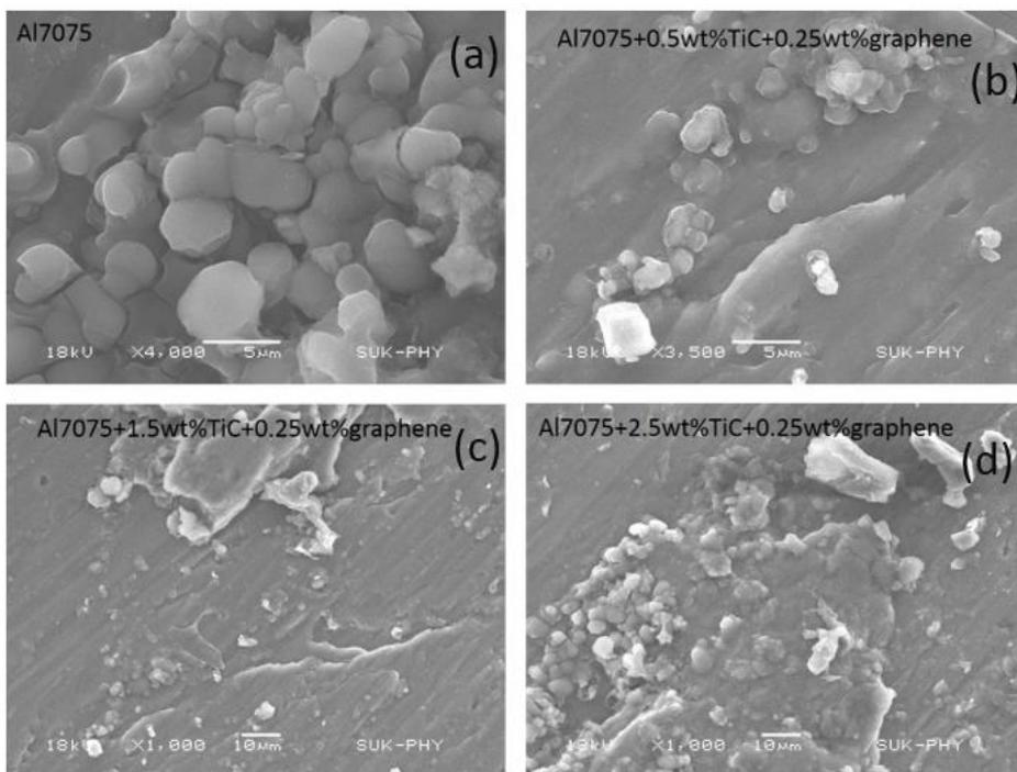
Fig. 4 SEM micrographs: (a) Al7075 alloy, (b-d) Al7075-TiC/graphene hybrid composites
