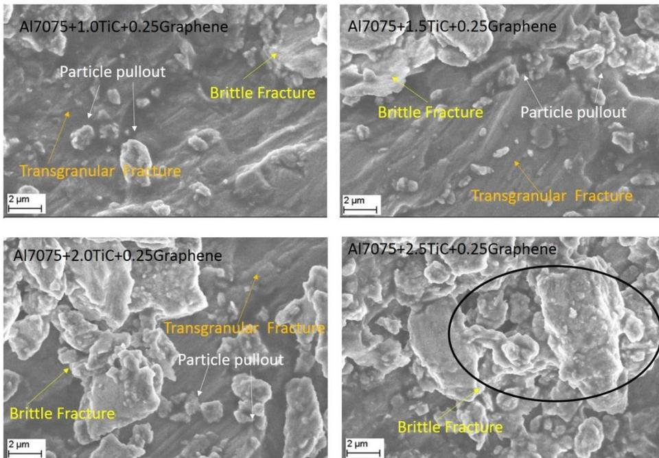
Fig. 7 SEM micrographs of the tensile fracture surface
