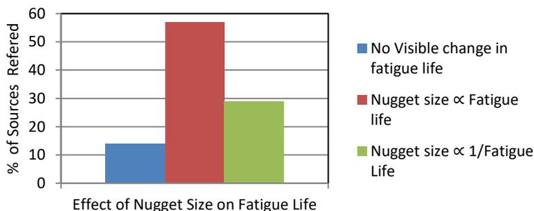
Fig. 3 Overview of effect of nugget size on fatigue life.
