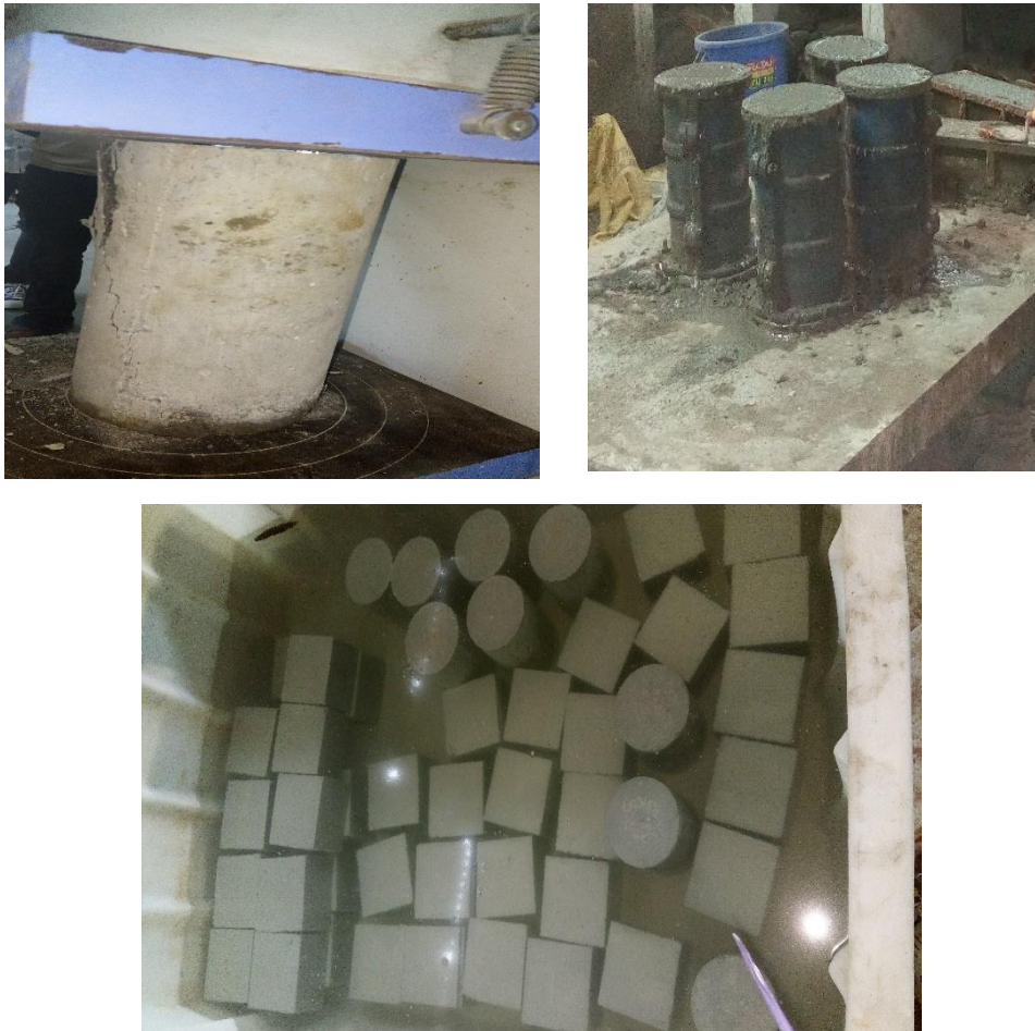
Fig. 2 shows a glimpse of experimental work that were subjected to compressive testing
