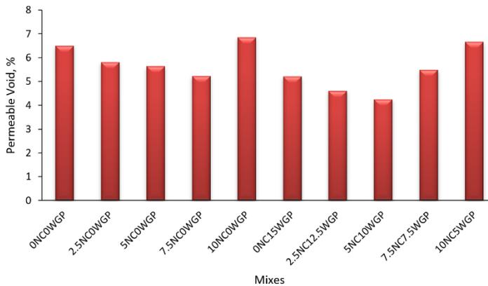
Fig. 23 Permeable voids % of all mixes
