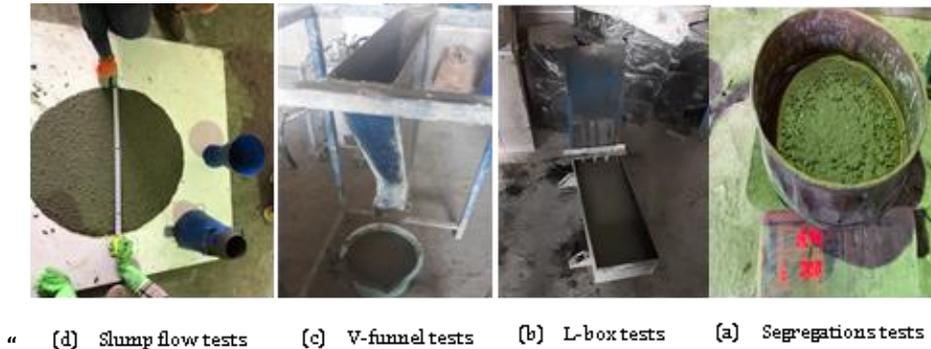
Fig. 7 Fresh Properties' Tests
