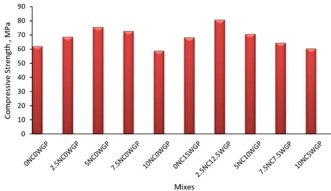
Fig. 15 Compressive strength for all SCC mixes
