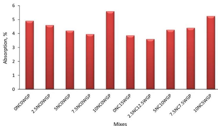
Fig. 22 Water absorption% of all mixes
