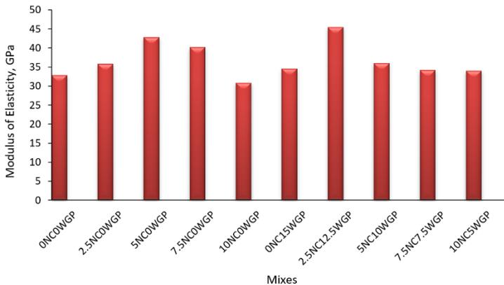
Fig. 16 Modulus of elasticity for all SCC mixes
