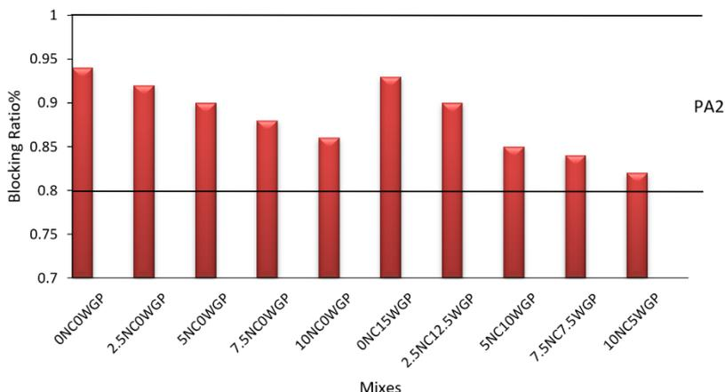
Fig. 13 Blocking ratio for all SCC mixes
