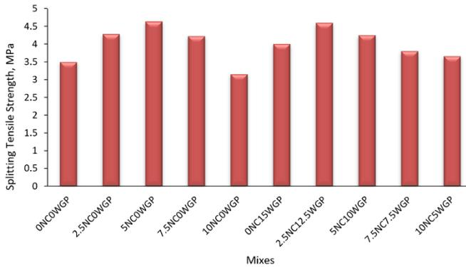
Fig. 19 Splitting strength for all SCC mixes
