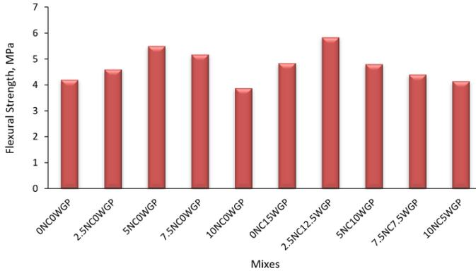
Fig. 18 Flexural strength for all SCC mixes
