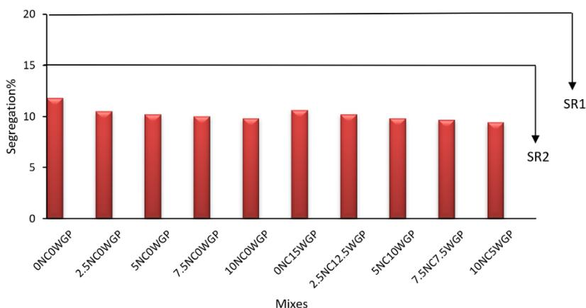
Fig. 14 Segregation ratio for all SCC mixes
