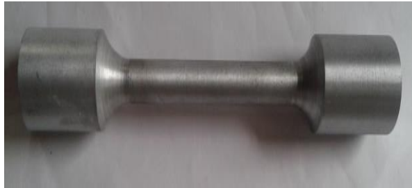
Fig. 4 Prepared tensile specimen as per ASTM standard E8
