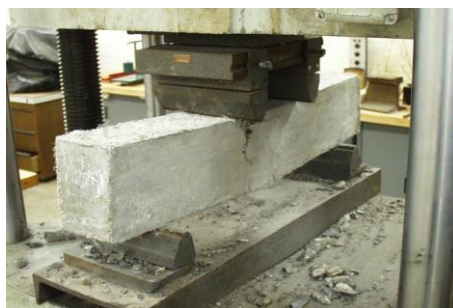
Fig. 11 Flexural test on beam
