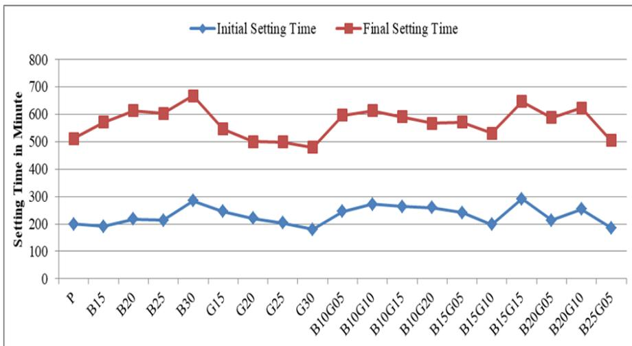
Fig. 2 Setting time for various binary and ternary mixes of SCBA & GGBFS
