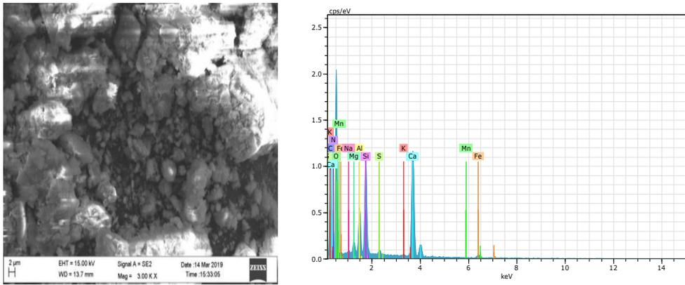
Fig. 9 SEM evaluation of concrete specimen using OPC by 30% GGBFS
