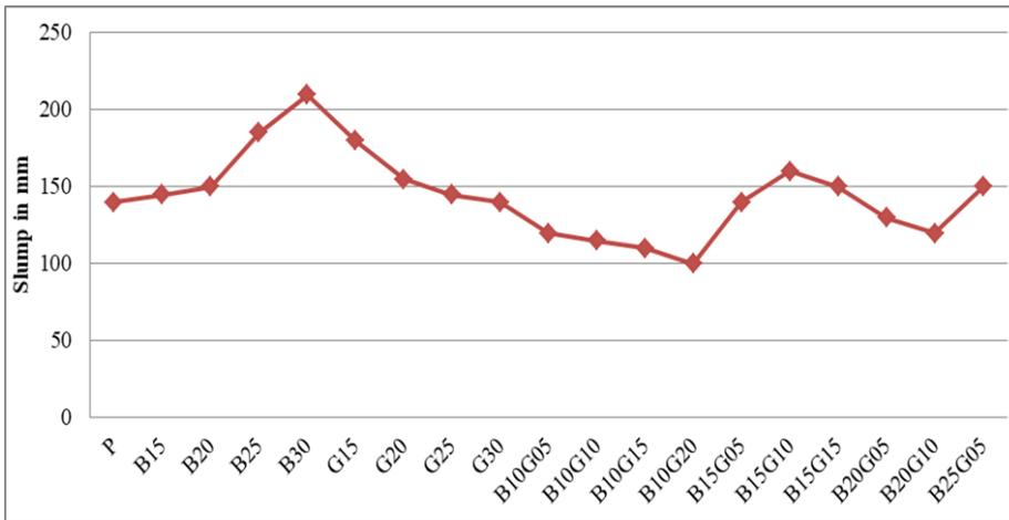
Fig. 1 Slump for various binary and ternary mixes of SCBA & GGBFS
