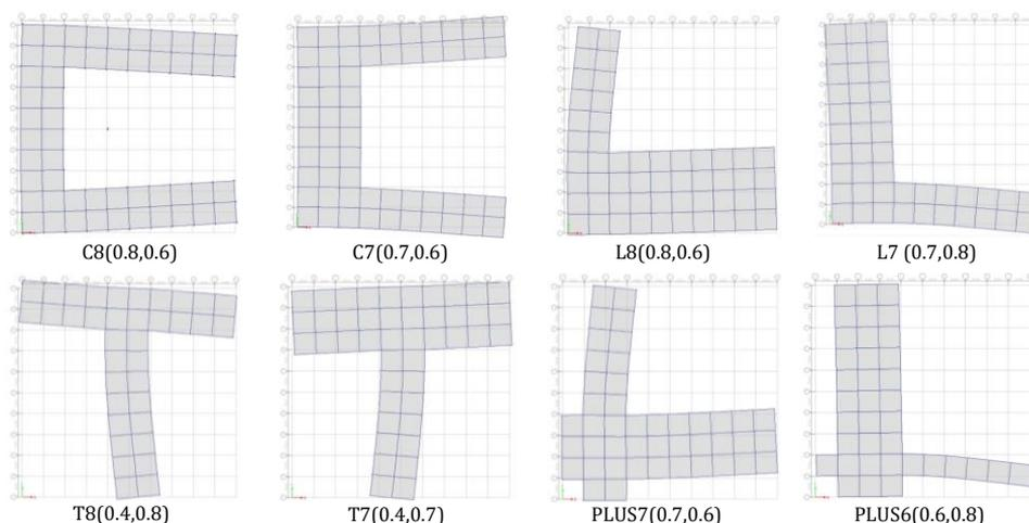
Fig. 6 Representative complicated deformed mode shapes of re-entrant RC building models
