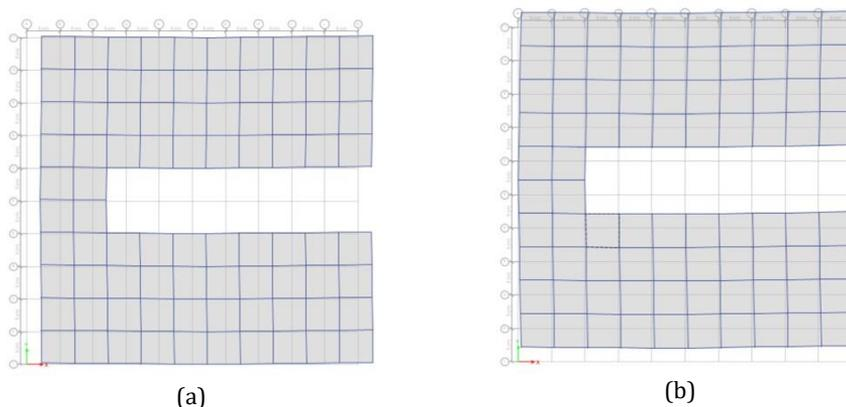
Fig. 8 Displacement profile in semi-rigid diaphragm
