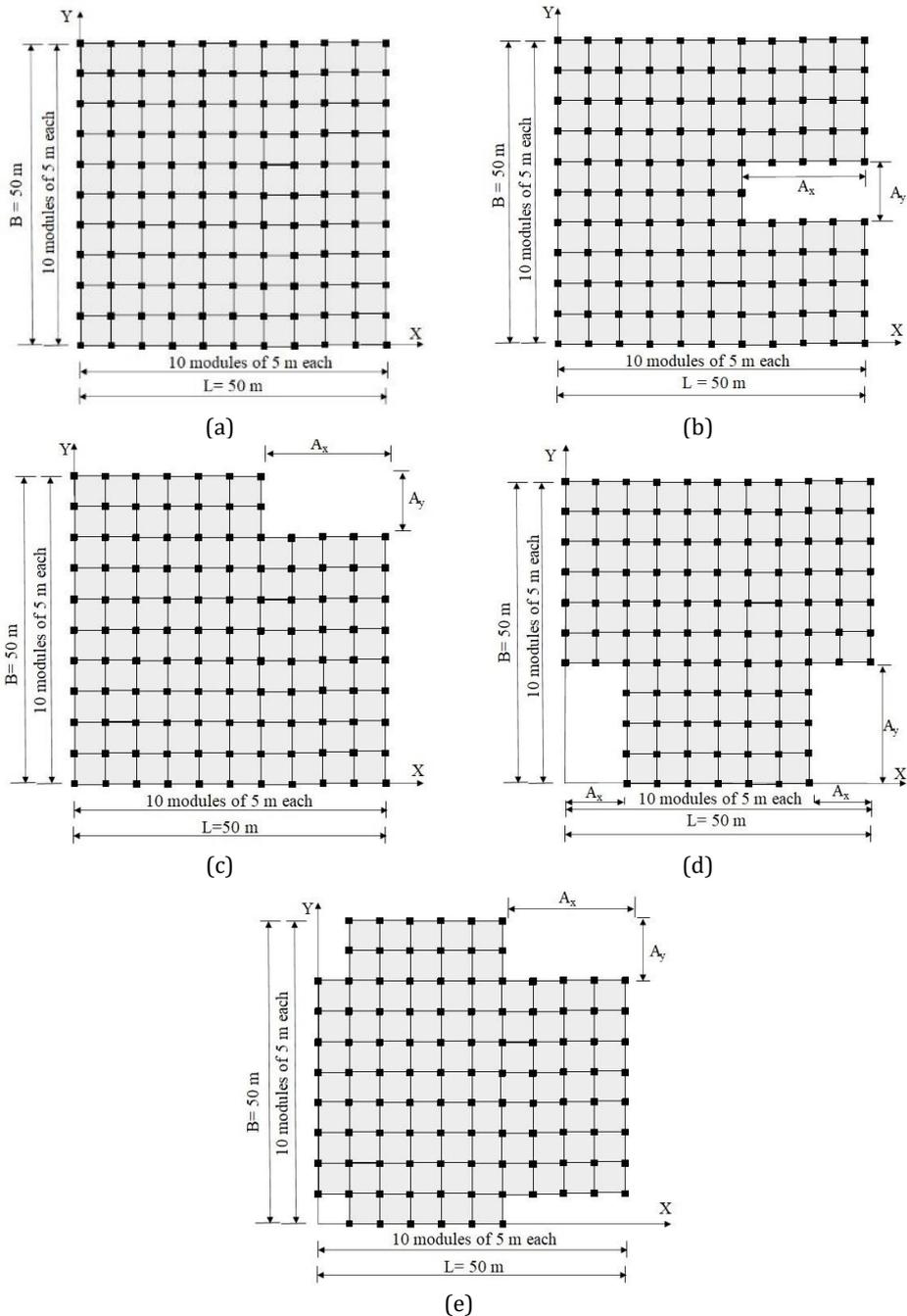
Fig. 2 Regular and plan irregular RC building models with  $A/L$  ratio 0.4 in the X-direction and 0.2 in the Y-direction, (a) Regular; (b) C-shaped; (c) L-shaped & (e) PLUS-shaped with  $A/L$  ratio 0.4 in the X direction and 0.2 in the Y-direction and (d) T-shaped with  $A/L$  ratio 0.2 in the X-direction and 0.4 in the Y-direction
