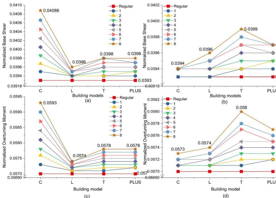
Fig. 4 (a) Normalized base shear response in X-direction for seismic force RSM-X; (b) Normalized base shear response in Y-direction for seismic force RSM-Y; (c) Normalized overturning moment response in X-direction for seismic force RSM-X and (d) Normalized overturning moment response in Y-direction for seismic force RSM-Y of regular and re-entrant dominant plan irregular RC building models
