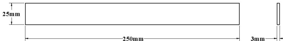
Fig 3. Solidworks drawing of tensile test sample
