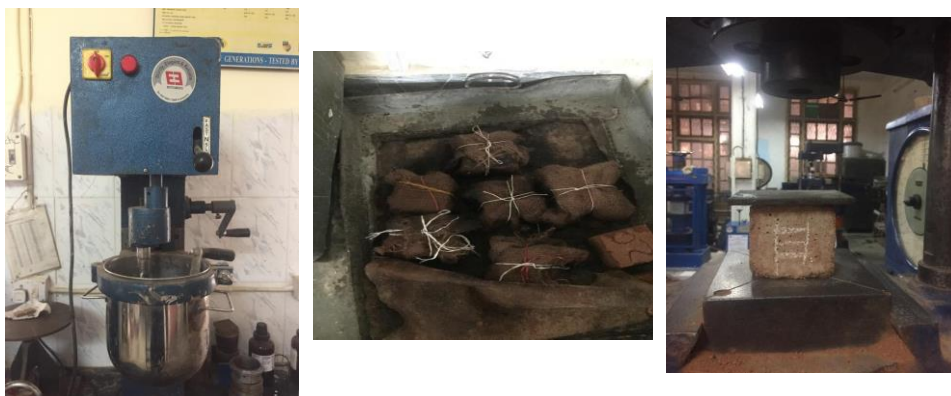
Fig. 3. (a) Mortar mixer, (b) curing of Lime mortar cube, and (c) UTM for compression test
