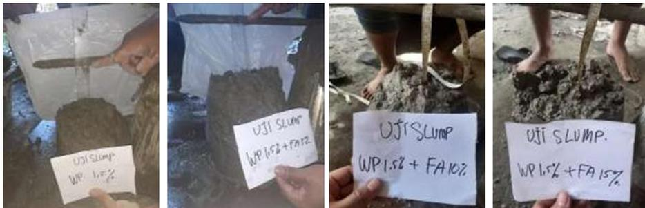
Fig. 3. Slump Abrams Test Measurement on BW, BWF1, BWF2, and BWF3
