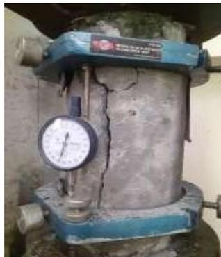
Fig. 7. The setting for testing modulus of elasticity
