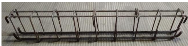
Fig. 2 Details of reinforcements of beam
