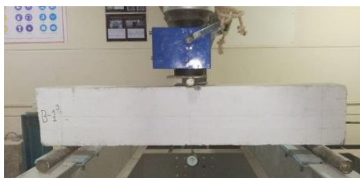
Fig. 6 Test setup and testing of beam
