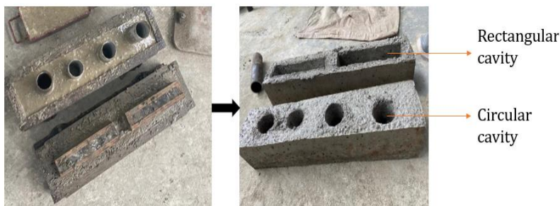
Fig. 3 Casting of RCB and CCB testing specimens for the study
