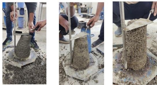
Fig. 7 Slump pattern of different concrete mix
