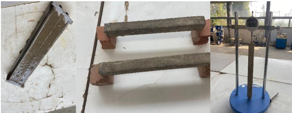
Fig. 5 Drying shrinkage test using length comparator
