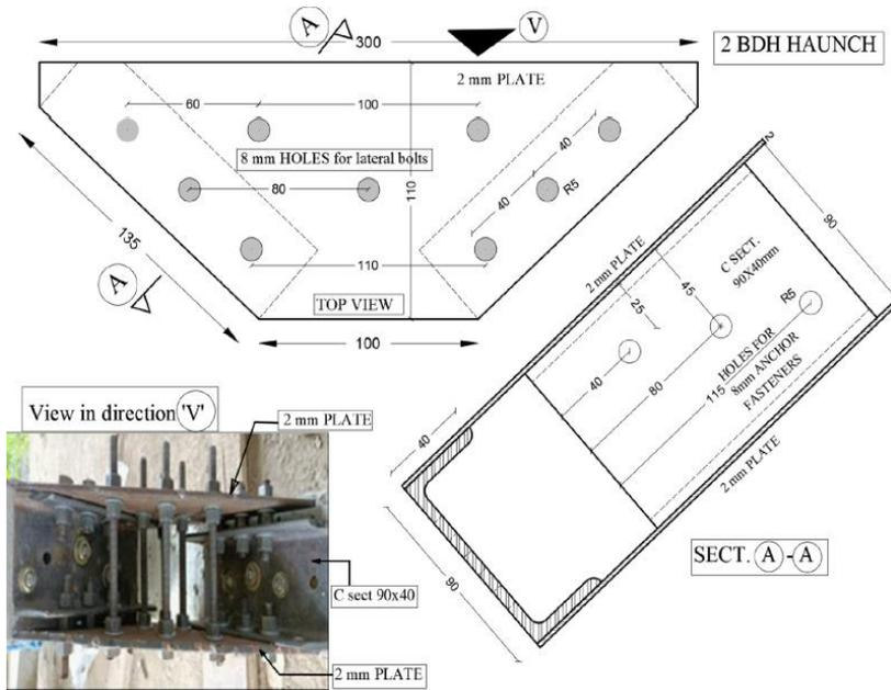
Fig. 14 Details of haunch used for experimental verification [39]
