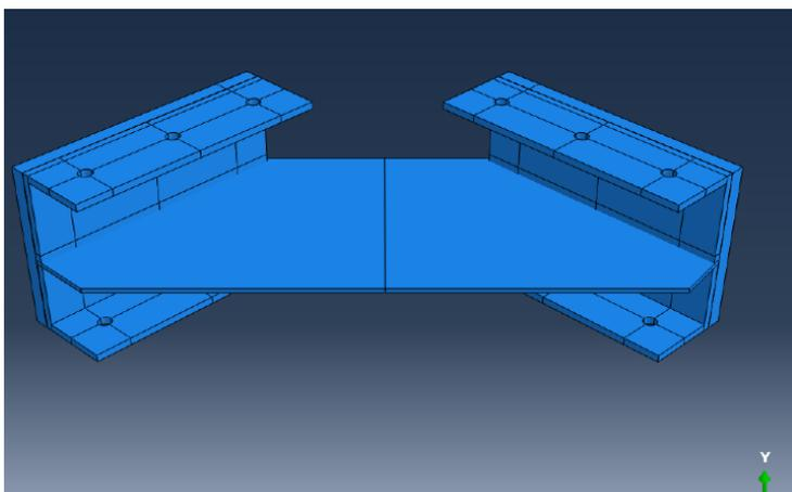
Fig. 8 Single Plate 8 mm tk. Welded Haunch
