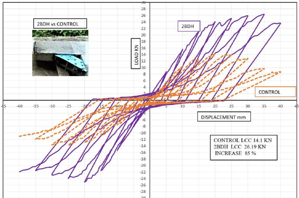
Fig. 15 Performance enhancement due to retrofit haunch [39]
