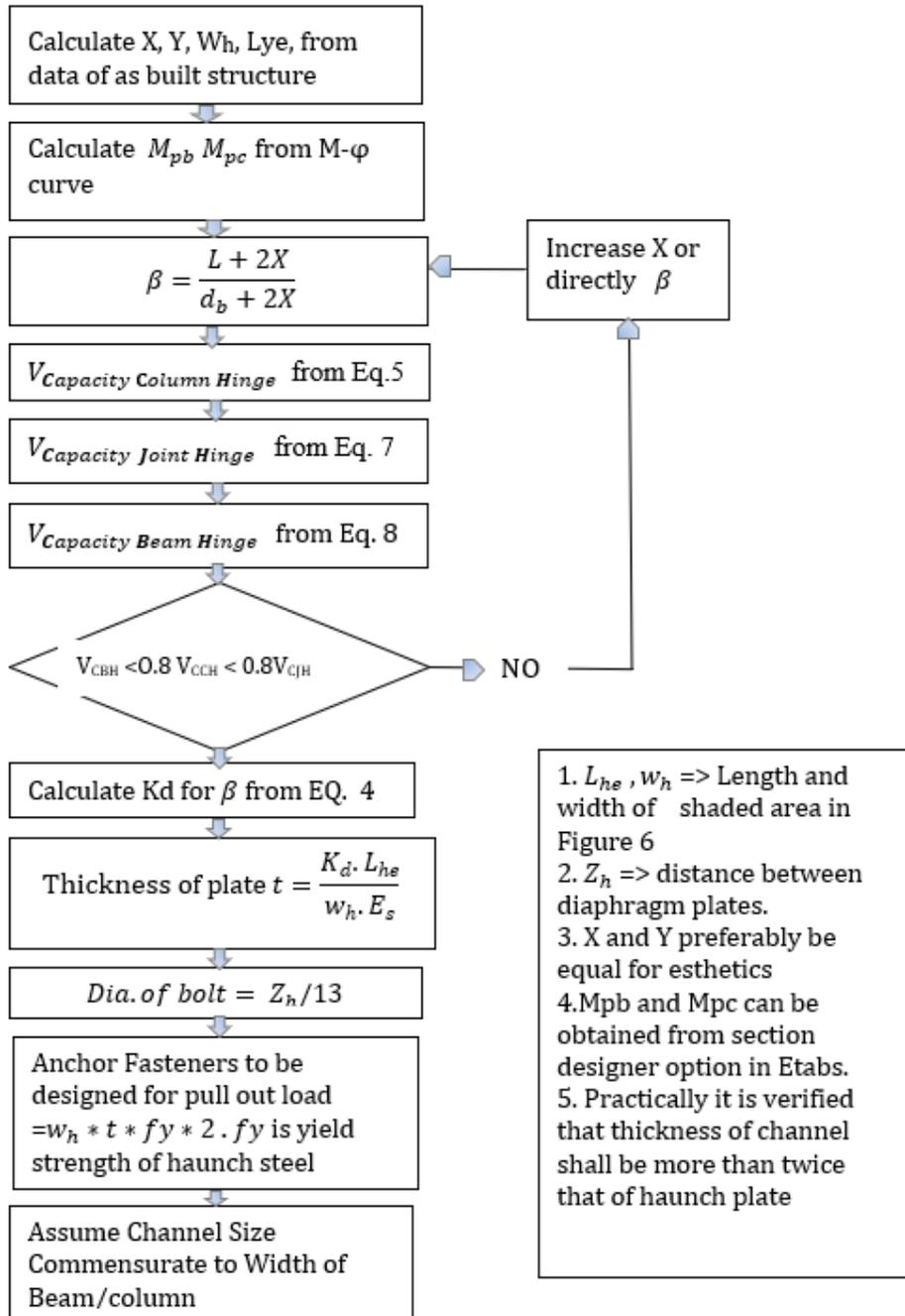
Fig.16 Flow Chart for Design of BDH Element
