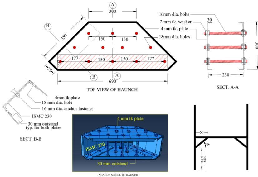
Fig. 7 Details of 4 BDH Haunch (4 BDH to indicate 4 mm thick haunch plates)
