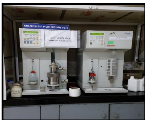
Fig. 1 Test setup for evaluation of pore structure
