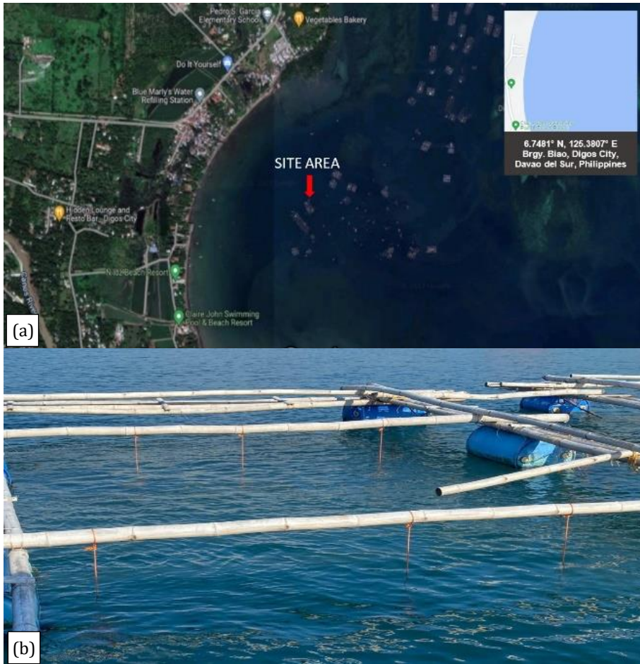
Fig. 3 Seawater environment in: (a) topographic view [19] and (b) actual curing condition of concrete cube samples
