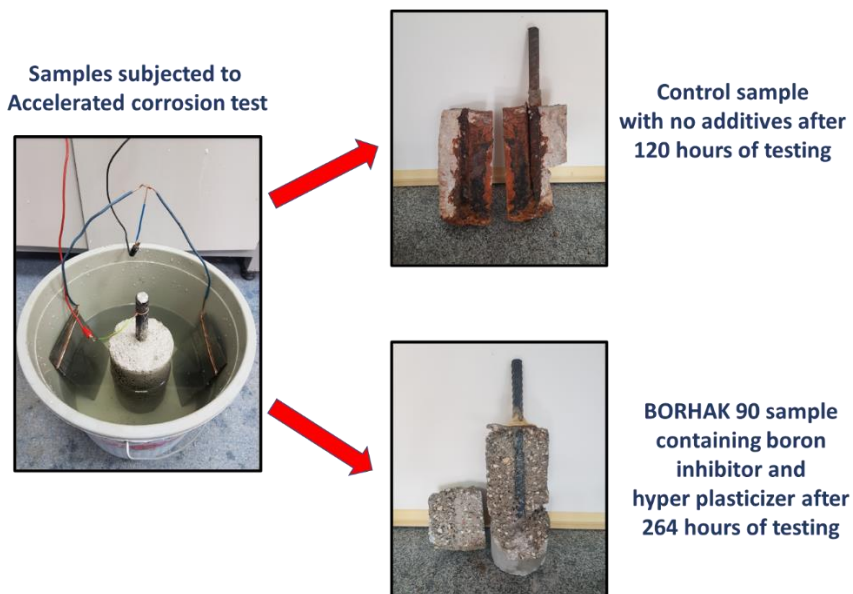
Fig. 7 Final stage of control and BORHAK sample after accelerated corrosion test
