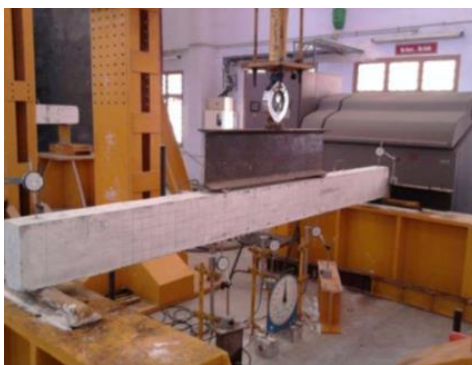
Fig. 7 Test Configuration for Flexure [52]
