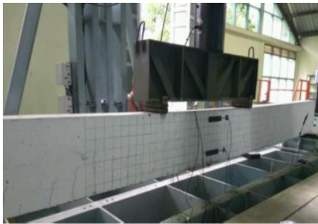
Fig. 5 Test Configuration for CRC beam Flexural Test [56]
