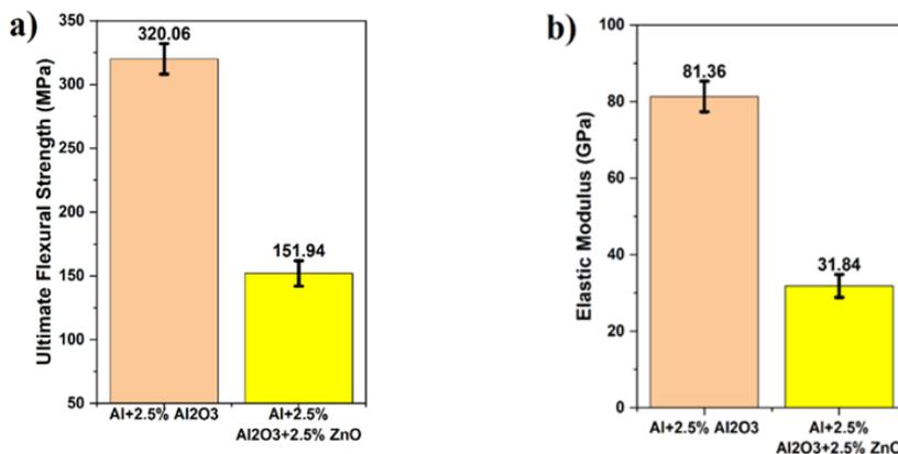
Fig. 11. (a) Ultimate Flexural Strength (UFS) and (b) Modulus of Elasticity (MoE) of Al MMC-01 and Al MMC-02
