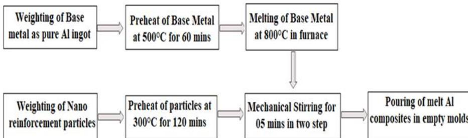
Fig. 4. Flowchart of the Stir casting process
