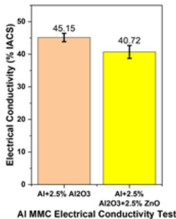
Fig. 13. Electrical Conductivity of developed two Al MMCs
