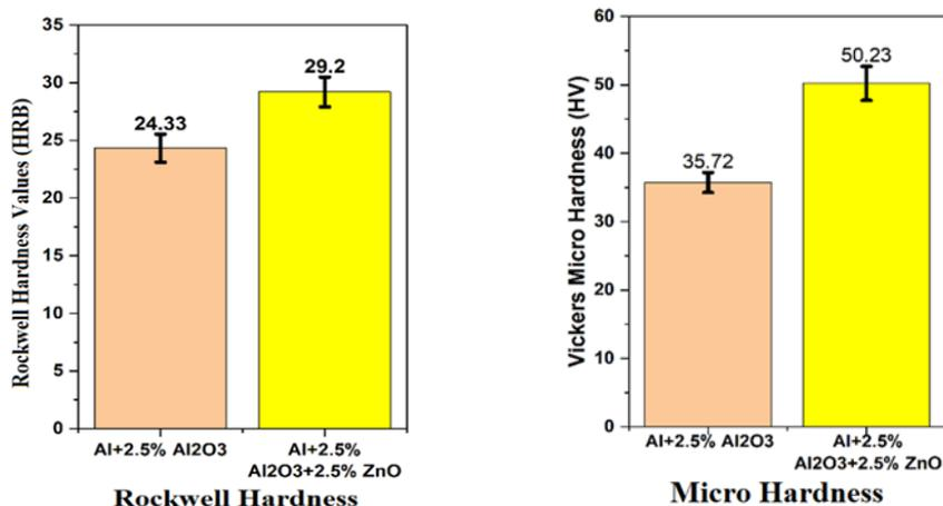
Fig. 9. Hardness test results of Al MMC-01 (Al+2.5% Al<sub>2</sub>O<sub>3</sub>) and Al MMC-02 (Al+2.5% Al<sub>2</sub>O<sub>3</sub>+ 2.5% ZnO)
