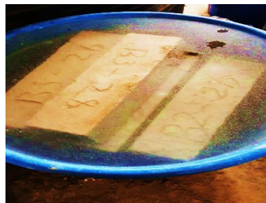
Fig. 2 Curing of beams by total immersion in water
