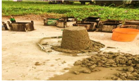
Fig. 3 Slump test on fresh concrete
