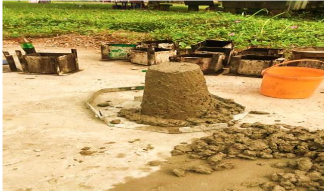
Fig. 3 Slump test on fresh concrete
