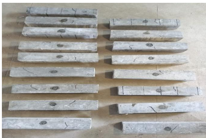
Fig. 2. Setup of cracked concrete specimens
