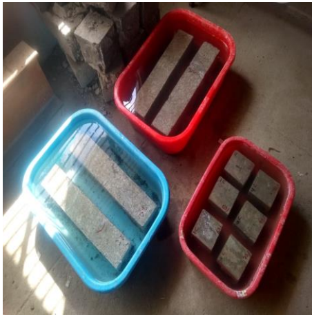
Fig.3 Concrete specimens cured at various curing agents
