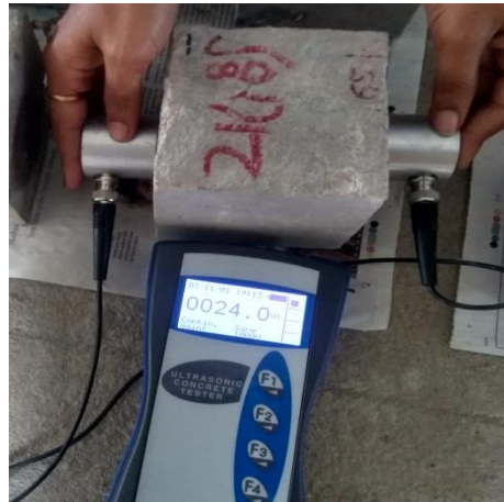
Fig.4 Setup of UPV measurement
